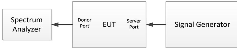
**Figure 2 – Uplink test configuration in EUT test mode**
