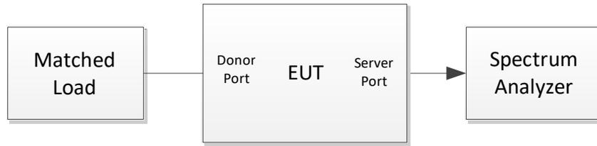
**Figure 6 – Maximum downlink noise limit test configuration**
