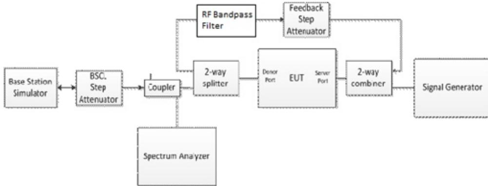
**Figure 10 – Uplink oscillation detection test setup**
