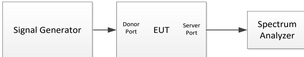
**Figure 3 – Downlink test configuration in EUT test mode**
