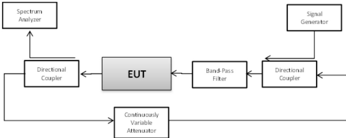
**Figure 13 – Mobile booster automatic feedback cancellation test procedure**
