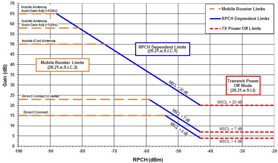
Figure D4 – Mobile provider-specific consumer signal booster variable gain limits
