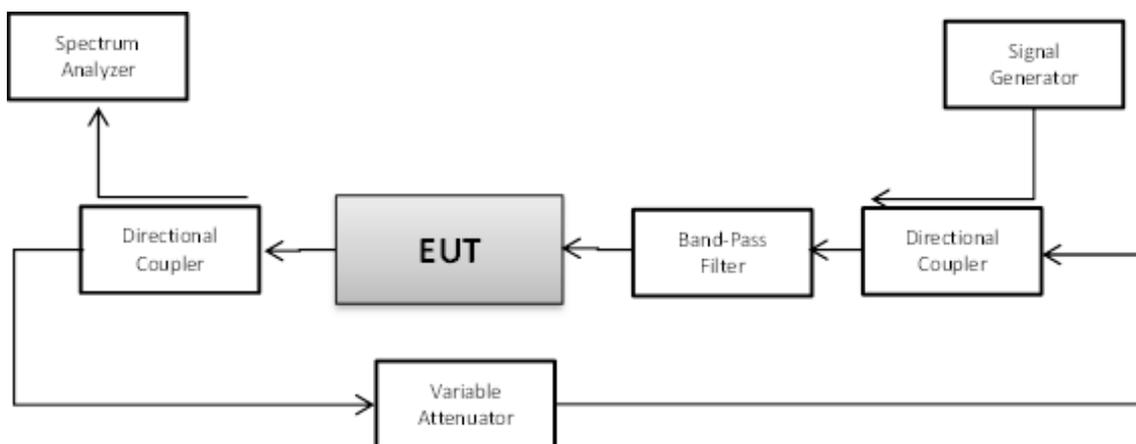
**Figure 12 – Downlink oscillation mitigation test setup**
