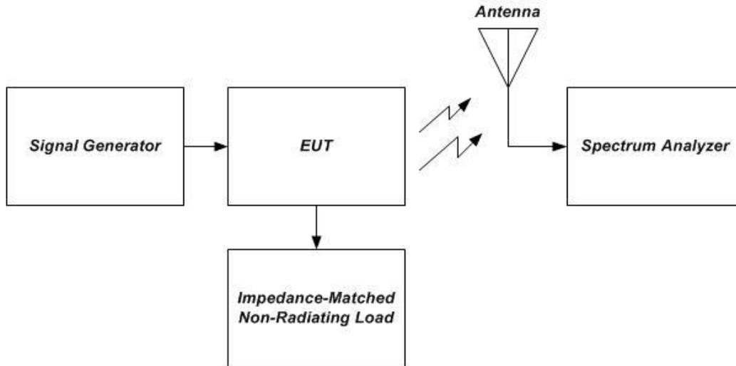
**Figure 14 – Radiated spurious emissions test instrumentation setup**
