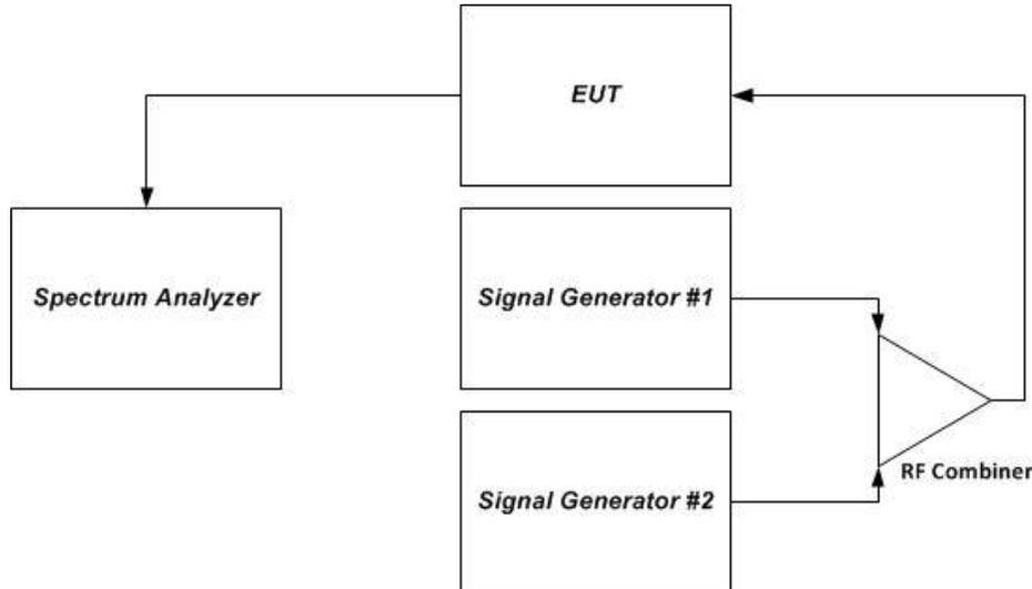
**Figure 5 – Intermodulation product instrumentation test setup**
