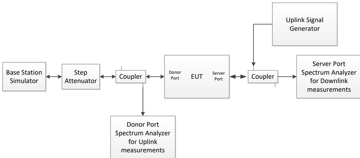
Figure 1 – Test configuration in EUT normal operational mode
