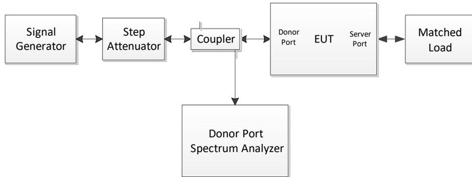
**Figure 7 – Uplink RSSI-dependent noise limit test configuration**
