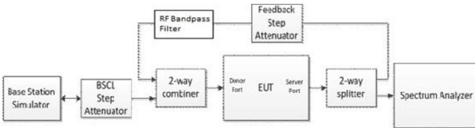
**Figure 11 – Downlink oscillation detection test setup**
