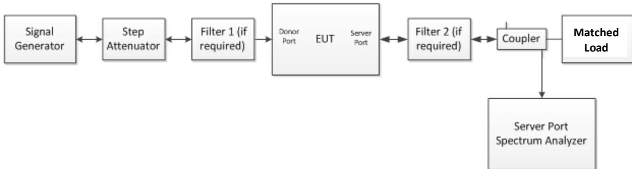
**Figure 8 – Downlink RSSI-dependent noise limit test configuration**
