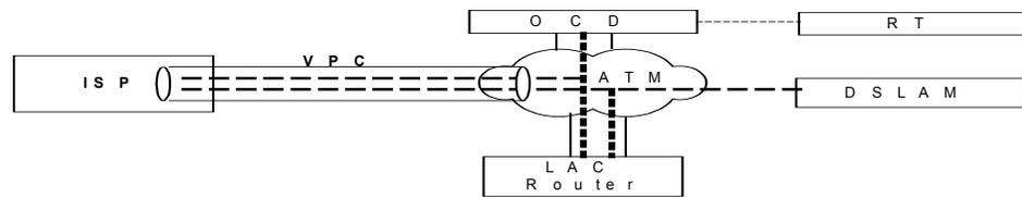
In the ASI-North Region, Layer Two Tunneling Protocol (L2TP) provisioning provides access to all DSLAMs in the LATA in which Customer requests Service. In cases where Company utilizes Optical Concentration Devices (OCDs) to connect to remote terminals (RTs) to provision DSL Transport, the same VPC also provides access to all remote terminals in the LATA.
