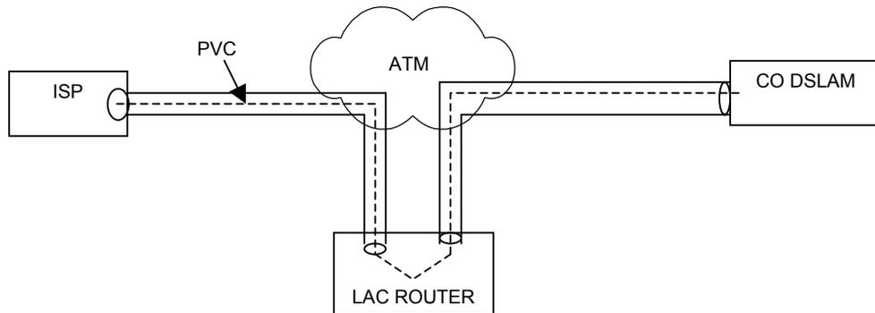
In the ASI-North Region, Layer Two Tunneling Protocol (L2TP) provisioning provides access to all DSLAMs in the LATA.
