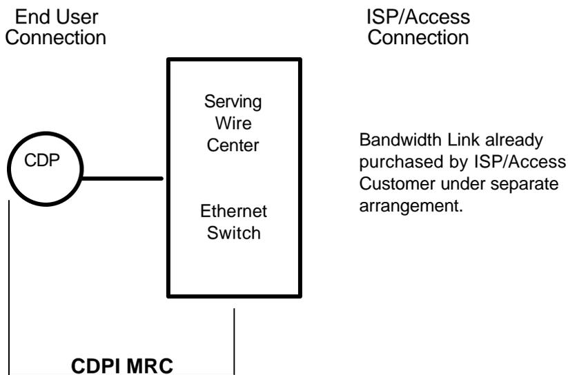
**METS Connection to ISP Interface (ISPI) at Ethernet Serving Wire Center**
