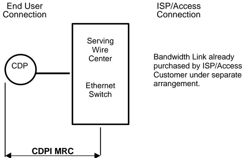
**METS Connection to ISP Interface (ISPI) at Ethernet Serving Wire Center**
