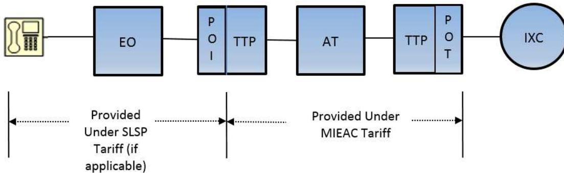
Note: The POI TTP and the POT TTP as shown in this diagram may be the same TTP or different TTPs.
