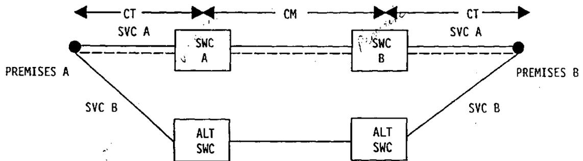
\_\_\_\_\_ Physical Routes for High Capacity Services A and B
