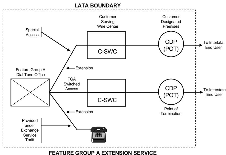
In the above example, two CDPs are utilized to better illustrate the concept. From a practical standpoint, both the Switched Access and Special Access Services could be routed via the same CDP.
