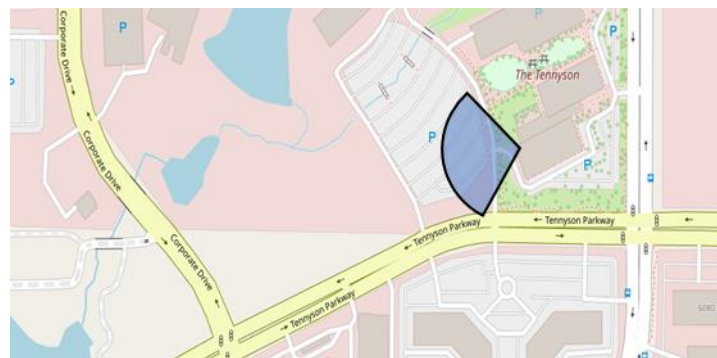
Figure 2: Tennyson Test Site. The transmitter will be placed at the corner of the building during testing. The test will take place across a section of parking lot and courtyard space. Azimuths for the beams may range from 315° to 195°.
