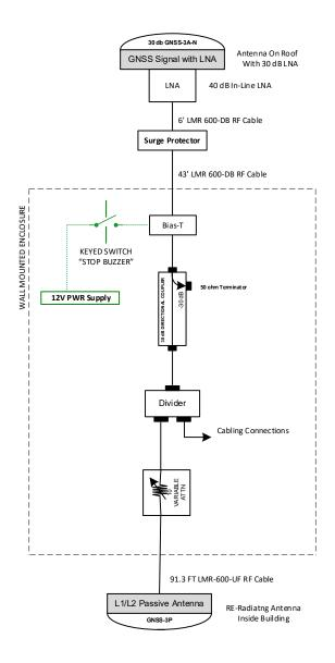
Figure 1, Building 60B Flight Test Bed Operations Lab Re-Radiator System
