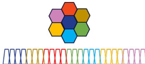
Figure 3 – Example of a seven frequency reuse pattern with a 5 megahertz channel (25 PRBs)
