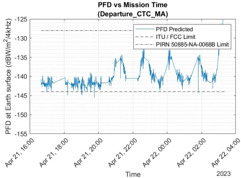
**Figure 11. NG-21 PFD during Departure Phase, TDRS MA (6M16G1D Emitter)**
