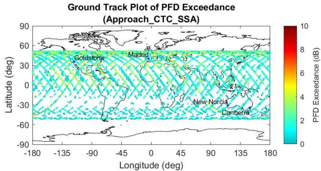
**Figure 17. NG-21 PFD Limit Exceedance during Mission Approach, TDRS SSA (6M16G1D Emitter)**
