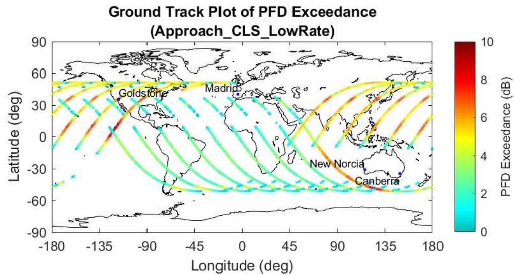
**Figure 21. NG-21 PFD Limit Exceedance during Mission Approach, CLS Low Rate (5M93G1D Emitter)**
