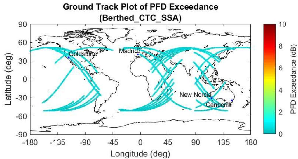
Figure 22. NG-21 PFD Limit Exceedance during Mission Berthed, TDRS SSA (6M16G1D Emitter)
