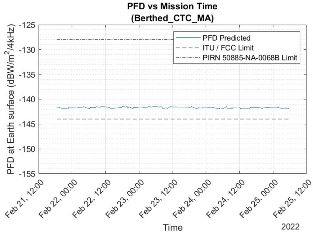
**Figure 7. NG-21 PFD during Berthed Phase, TDRS MA (6M16G1D Emitter)**
