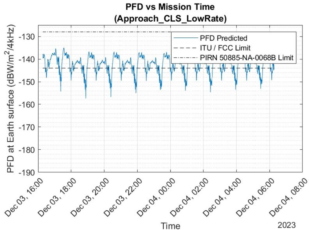
**Figure 5. NG-21 PFD during Approach, CLS Low Rate (5M93G1D Emitter)**
