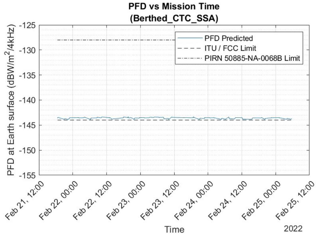
**Figure 6. NG-21 PFD during Berthed Phase, TDRS SSA (6M16G1D Emitter)**
