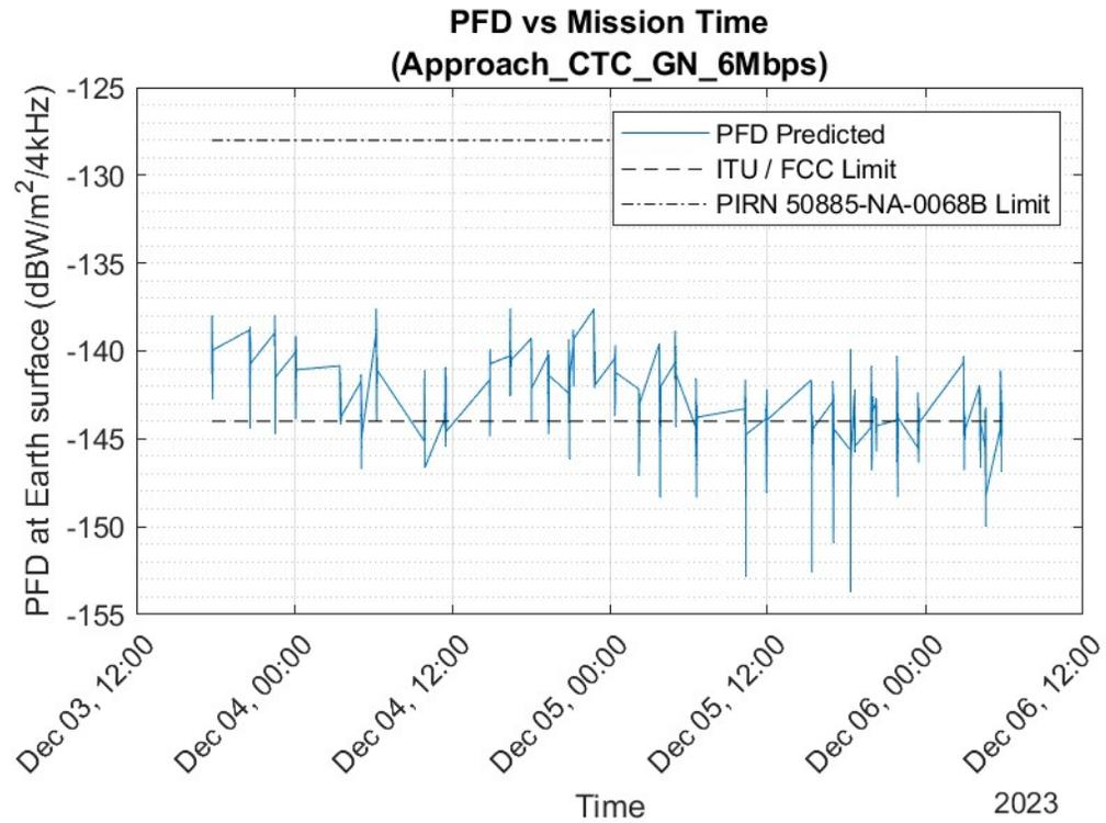
**Figure 3. NG-21 PFD during Approach, GN 6 Mbps (4M98G1D Emitter)**
