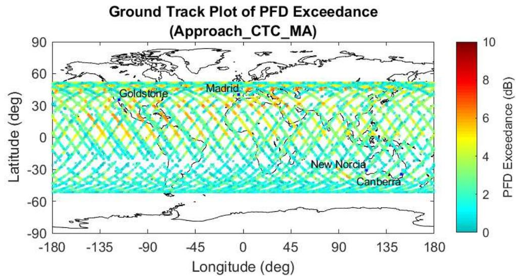
Figure 18. NG-21 PFD Limit Exceedance during Mission Approach, TDRS MA (6M16G1D Emitter)
