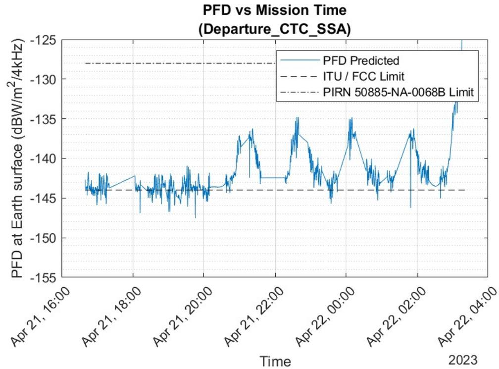
Figure 10. NG-21 PFD during Departure Phase, TDRS SSA (6M16G1D Emitter)
