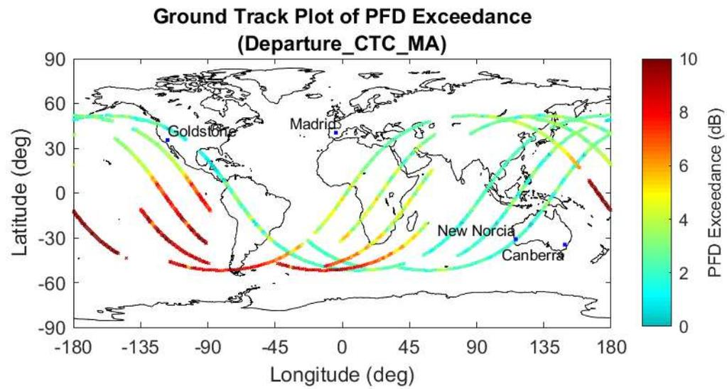
Figure 27. NG-21 PFD Limit Exceedance during Mission Departure, TDRS MA (6M16G1D Emitter)
