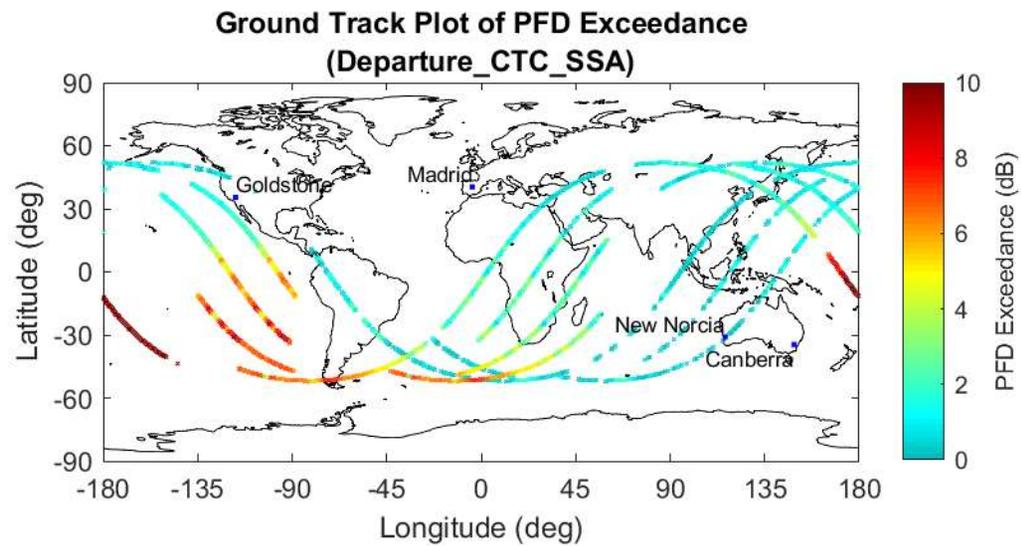
Figure 26. NG-21 PFD Limit Exceedance during Mission Departure, TDRS SSA (6M16G1D Emitter)
