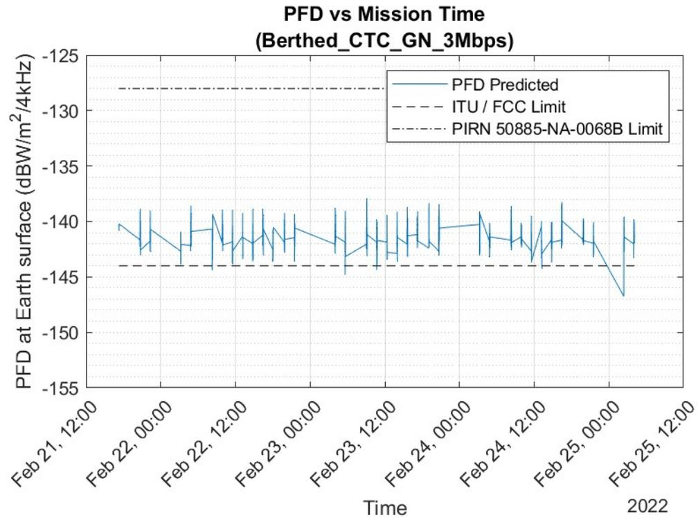
**Figure 9. NG-21 PFD during Berthed Phase, GN 3Mbps (3M00G1D Emitter)**
