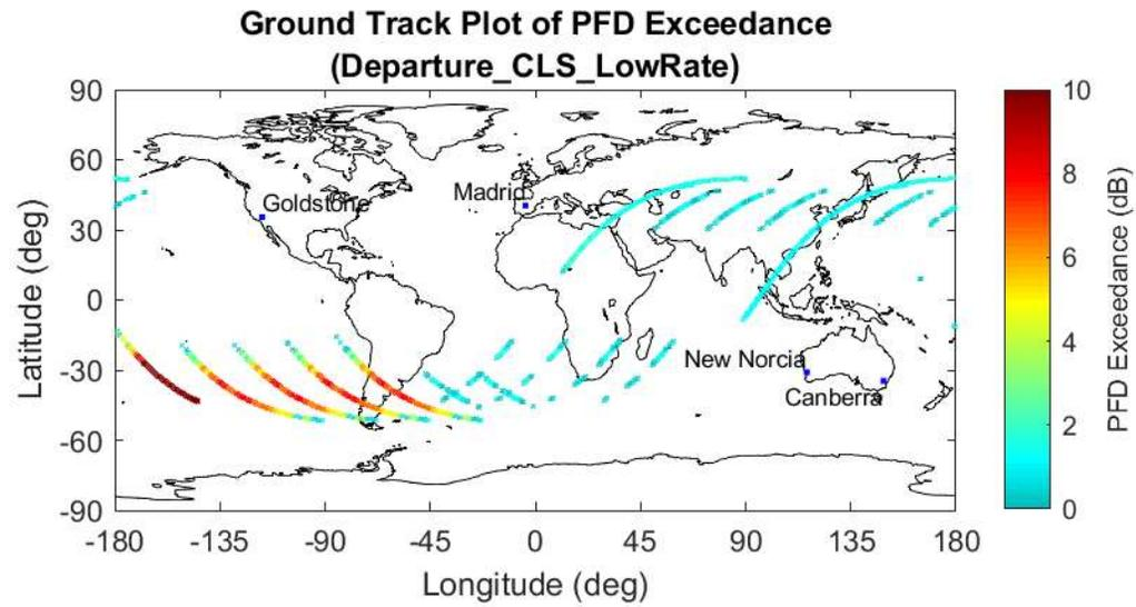
Figure 30. NG-21 PFD Limit Exceedance during Mission Departure, CLS Low Rate (5M93G1D Emitter)
