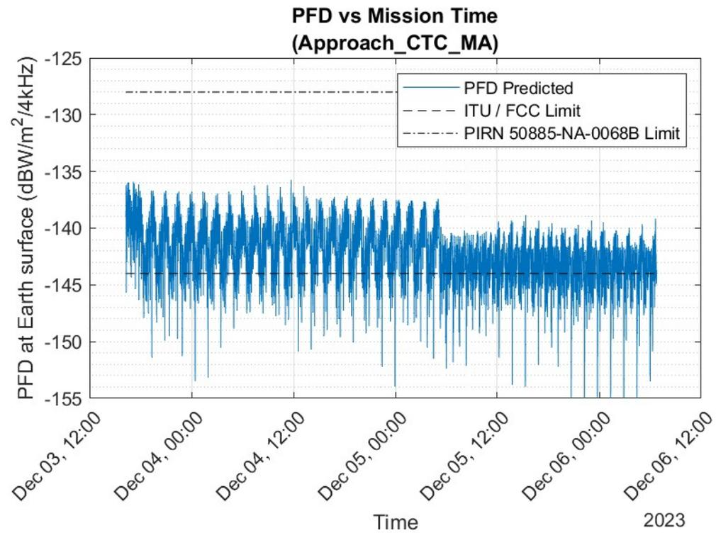
Figure 2. NG-21 PFD during Approach, TDRS MA/SMA (6M16G1D Emitter)
