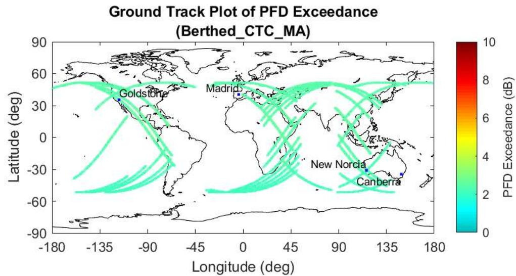
Figure 23. NG-21 PFD Limit Exceedance during Mission Berthed, TDRS MA (6M16G1D Emitter)
