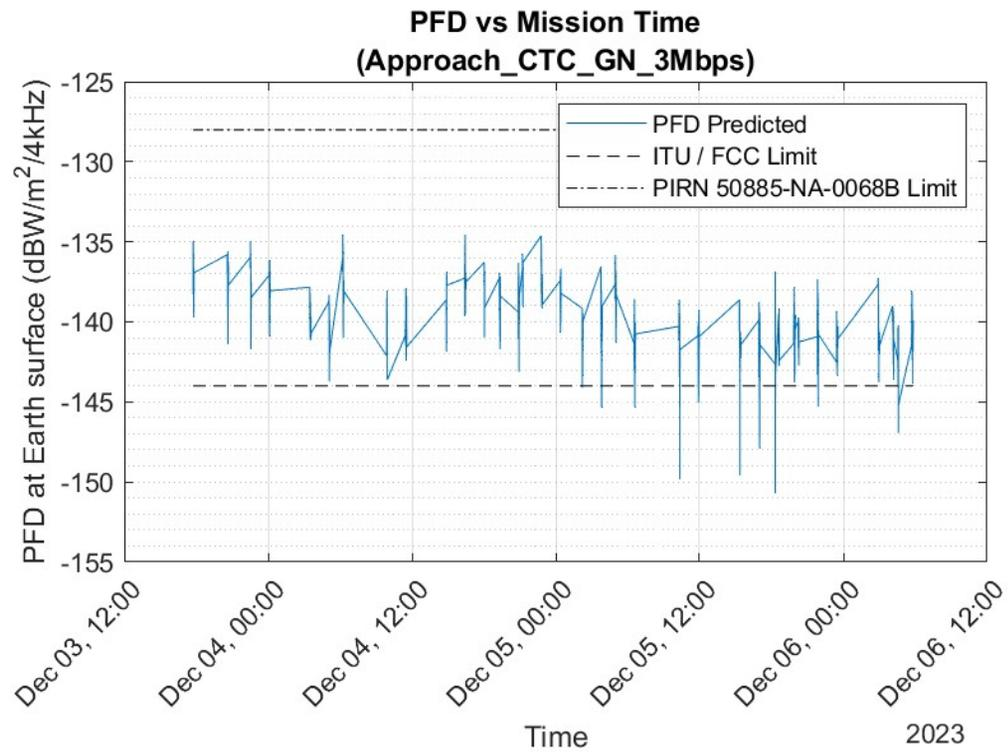
**Figure 4. NG-21 PFD during Approach, GN 3Mbps (3M00G1D Emitter)**
