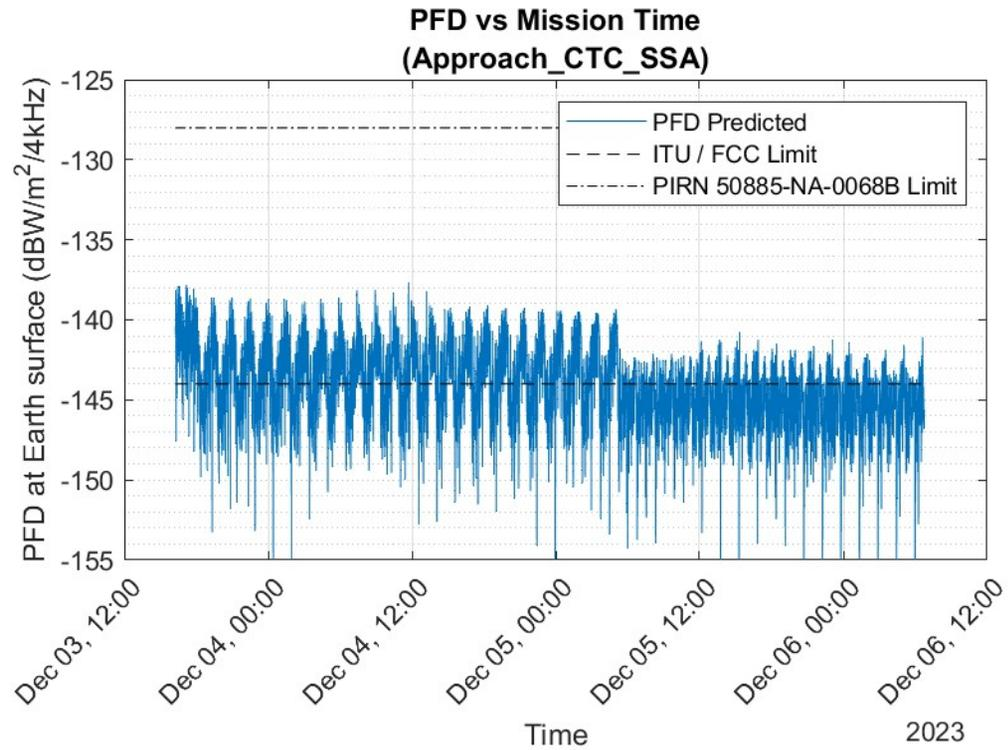
**Figure 1. NG-21 PFD during Approach, TDRS SSA (6M16G1D Emitter)**
