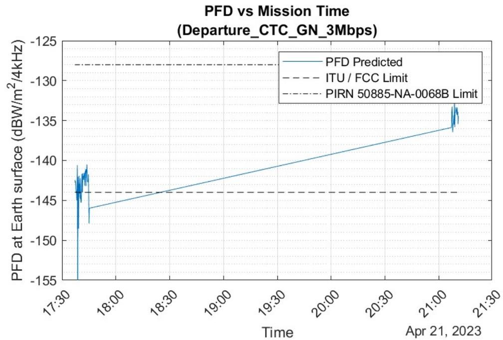
Figure 13. NG-21 PFD during Departure Phase, GN 3 Mbps (3M00G1D Emitter)
