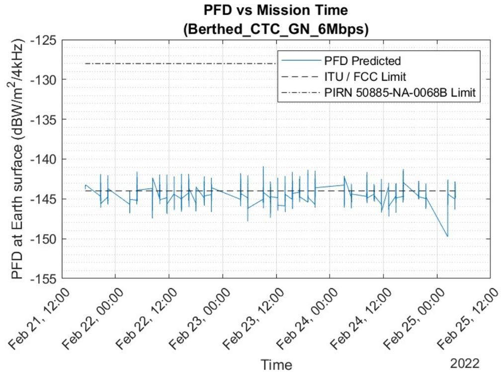
Figure 8. NG-21 PFD during Berthed Phase, GN 6 Mbps (4M98G1D Emitter)
