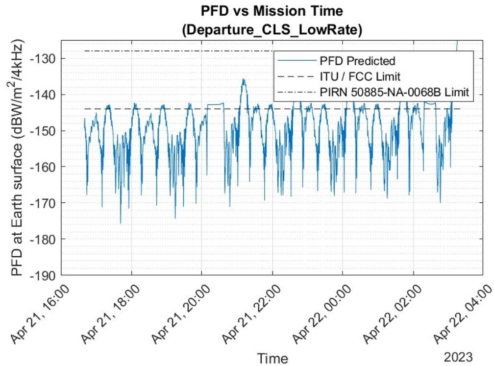
**Figure 14. NG-21 PFD during Departure Phase, CLS Low Rate (5M93G1D Emitter)**
