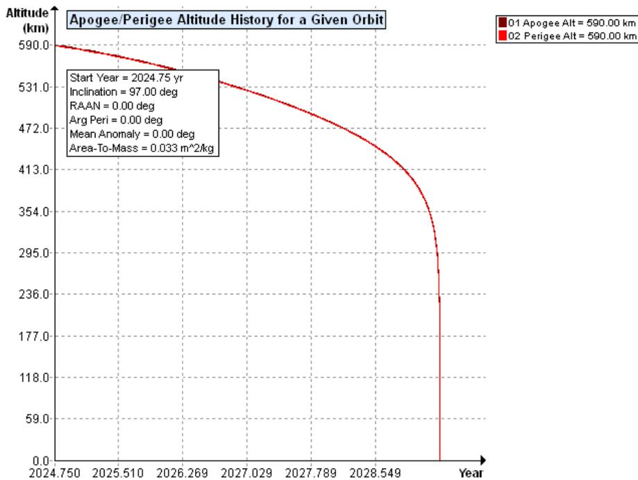
**Figure 2. Altitude vs. Time For Veery-0F Spacecraft Starting at 590 km Orbit. Obtained Using NASA DAS 3.2.6. See Appendix A for More Details.**
