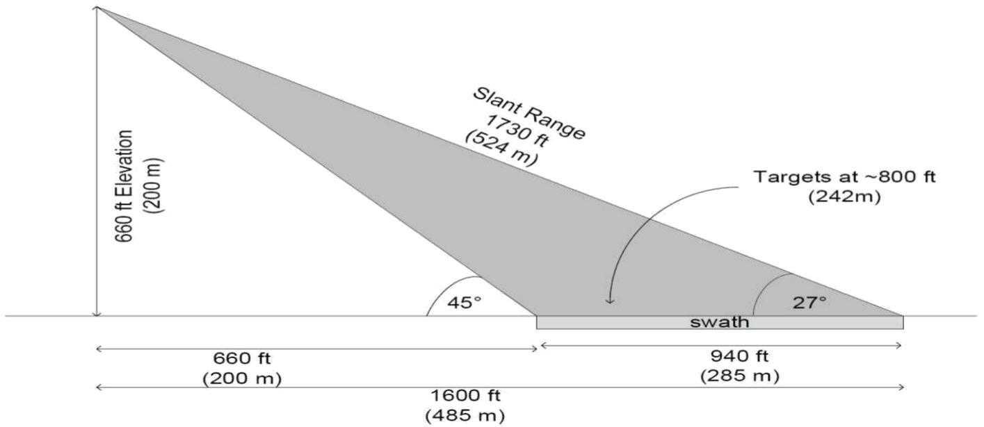
**Figure 2. Example SAR geometry, from an airborne platform.**
