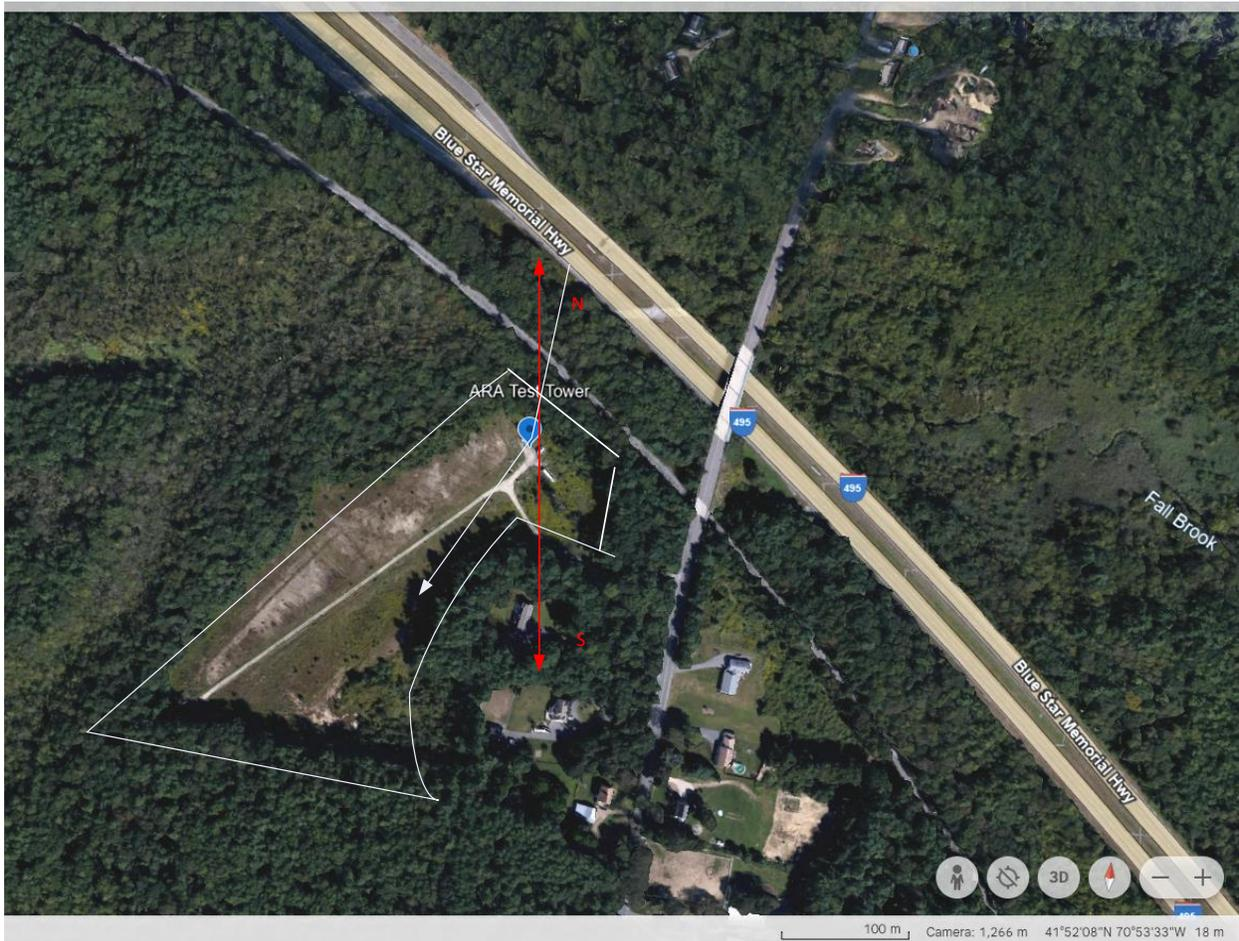
Figure 2 ARA Test Range, boundary, Azimuth Angle of Transmission scan in Azimuth clockwise from 221 deg true N to 15 degs true N)
