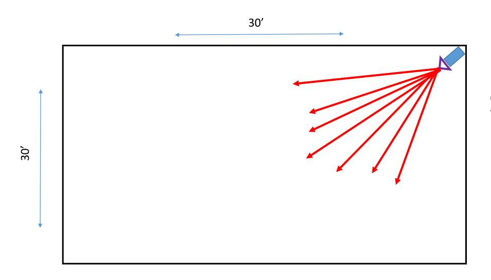
\*External Antenna connected to amp via 100 ft. LMR-400
