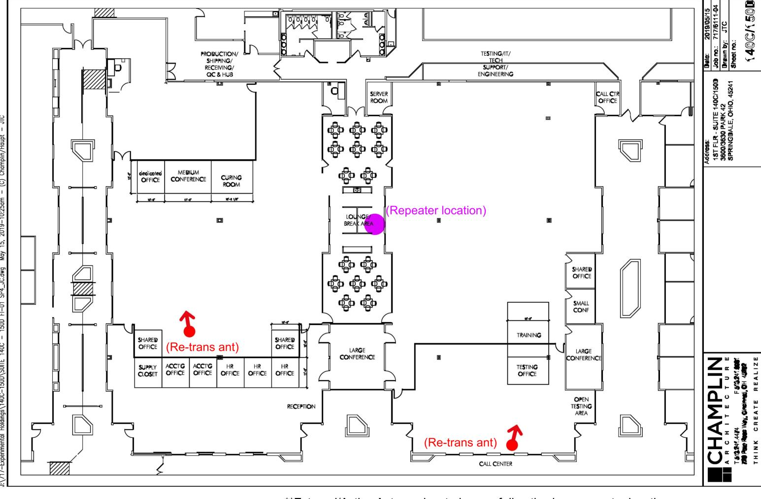
\*\*External/Active Antenna located on roof directly above repeater location. 100 ft. of LMR-240 connecting antenna and repeater.
