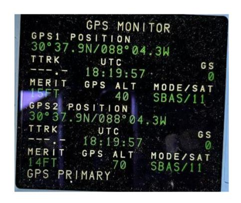
Flight Line Dock 7, Local Time 13:19 - 13:30 GPS PRIMARY GPS1 MODE initially NAV, then SBAS GPS1 Position Data valid GPS2 MODE initially NAV, then SBAS GPS2 Position Data valid
