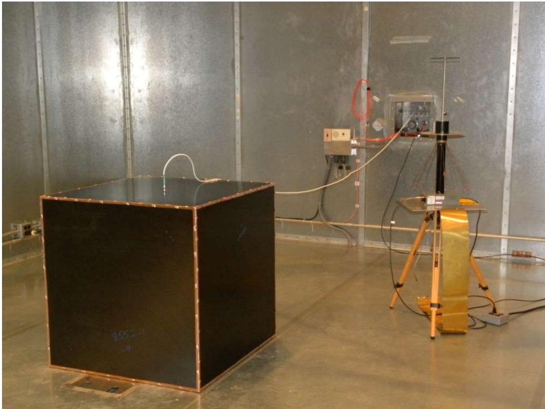
Taped composite box on metal floor, EMI antenna @ 1 meter distance
