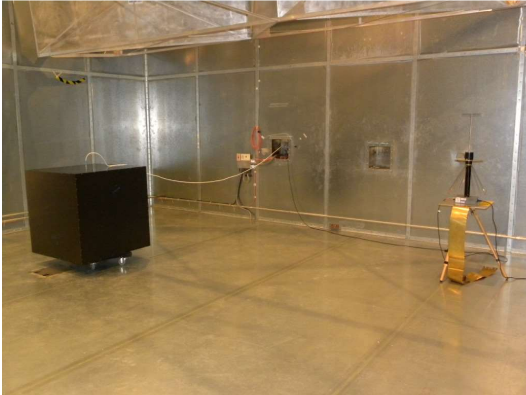
Composite box isolated from metal floor, EMI antenna @ 3 meters distance
