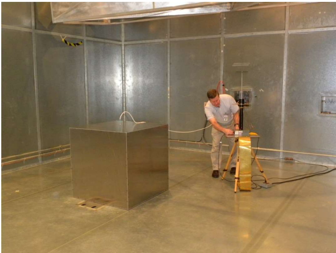
Aluminum box on metal floor, EMI antenna @ 1 meter distance
