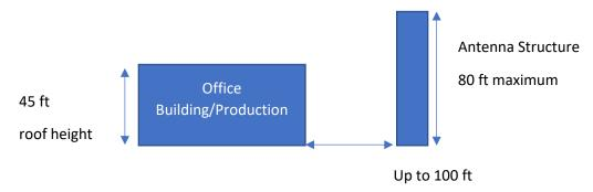
Position of tower when mounting radar will always maintaining safety limits
