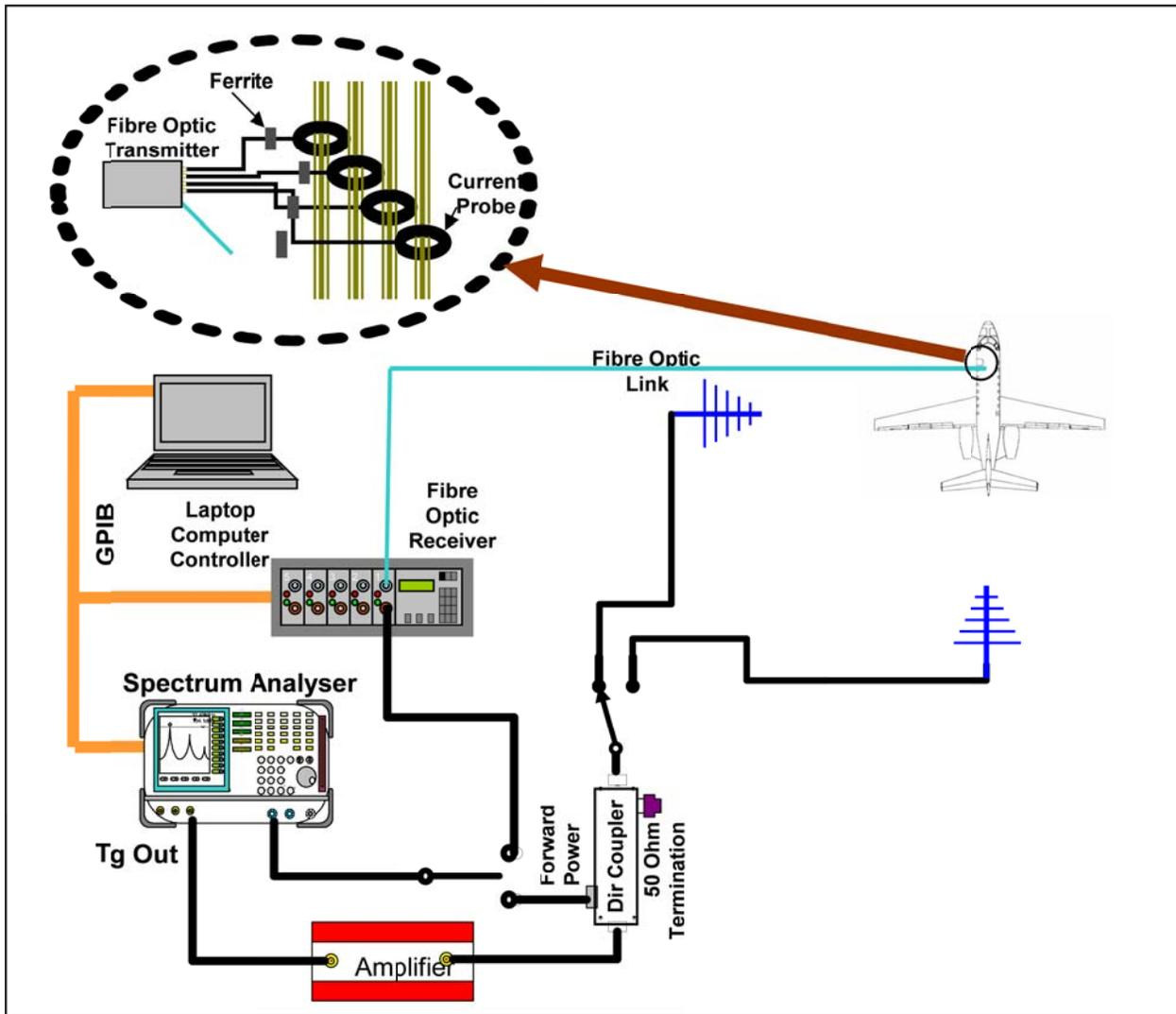
Figure 3 – LLSC Test Set-up Schematic
