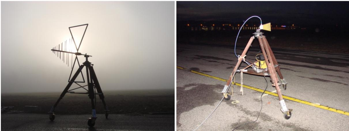
Figure 6 – LLSF antennas – Bi-Log and Double-Ridged Guide Horn
