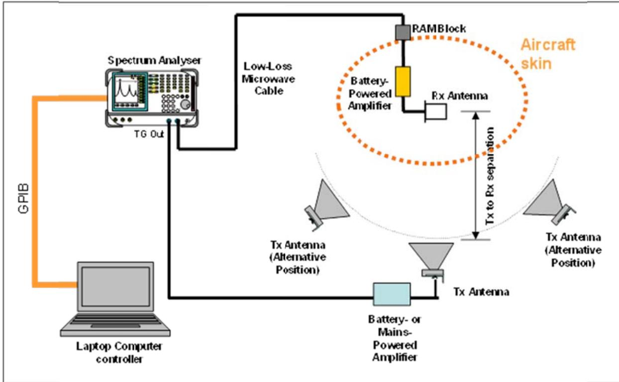
Figure 7 – LLSF Test Set-up Schematic
