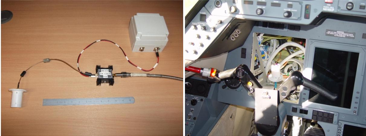
Figure 5 – LLSF Receive Antenna (Above 1 GHz) & Battery-powered Pre-amplifier
