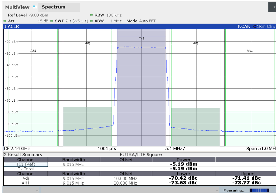
Measured ACPR for a 10 MHz LTE test model E-TM1_1
