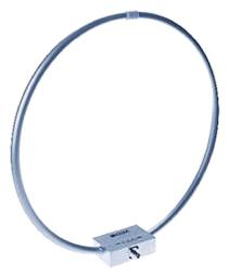
ETS-Lindgren's Model 6512 has a frequency range of 9 kHz - 30 MHz and is a passive loop antenna designed for both EMC emissions and EMC immunity tests. Every loop antenna can be individually calibrated in accordance with ANSI C63.5, using NIST traceable equipment. By knowing the actual antenna factors and performance characteristics of an antenna instead of typical data, you can more accurately measure field strength in your tests.
