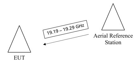
The EUT will be operated in a receive-only capacity throughout the testing.
