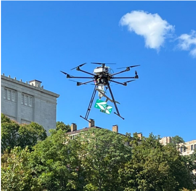
1486-EX-ST-2022 Exhibit #3, additional photos of radar mounted on small multi-rotor drone
