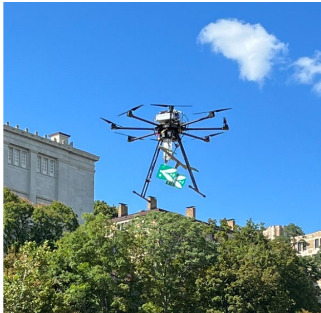
Low-power radar flying on a Tarot X8 drone.
