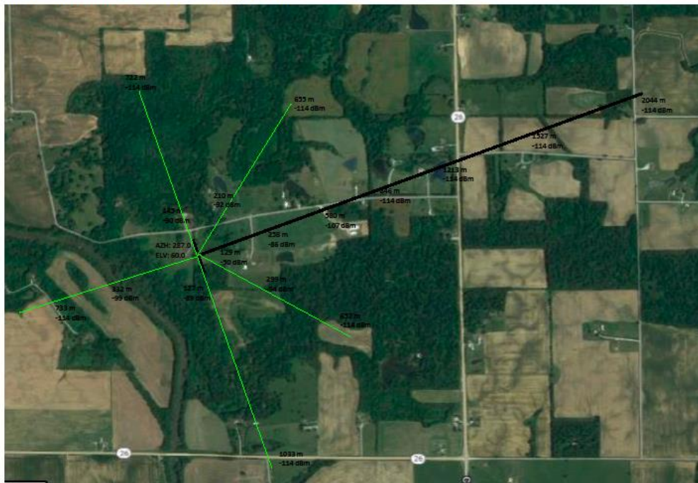
Figure 1 Signal Strength Measurements for NSL Ground Station Antenna
