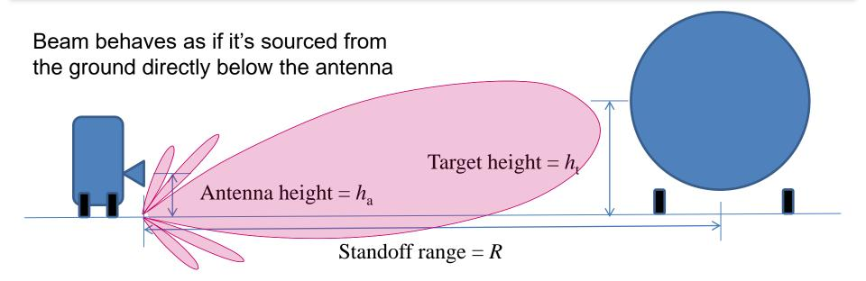
Calculation to ensure the ground-bounce peak beam is on the target
