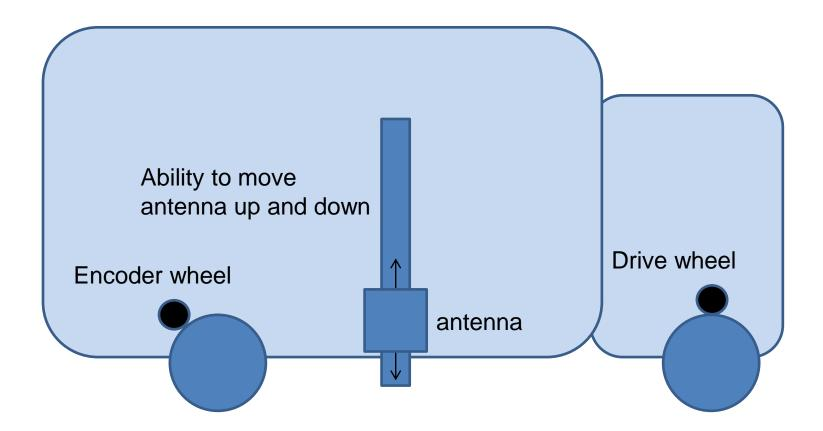
Drive wheel is used to move the truck (via friction) at a slow and constant pace (i.e., no one driving and riding the brakes). Encoder wheel is separate and serves to tell the radar how far the truck has moved.
