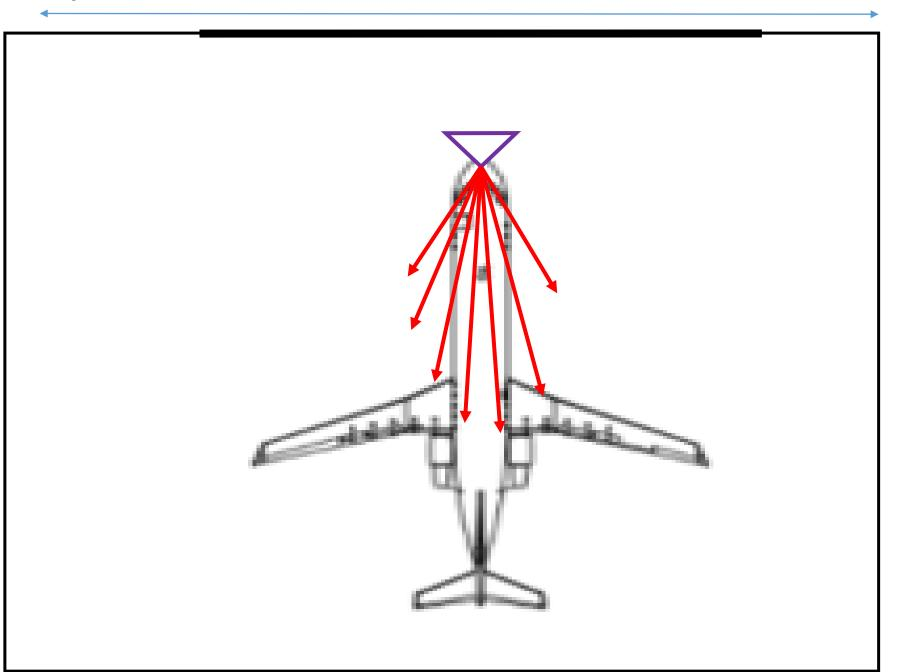
External Antenna located directly above amplifier, connected via 100 ft. of LMR-240
