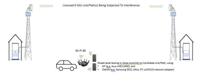
Figure-1: Sample of Outdoor Test Setups
