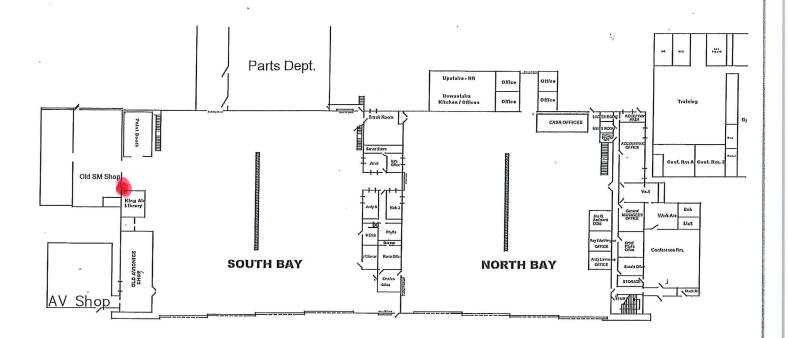
Hanger Floor Plan Aero Contractors 3463 Swift Creek Road Smithfield, NC, 27577 GPS reradiate antenna will be placed at the mezzaine level of the south wall in the southern bay, above the King Air library. (see red dot) 6
