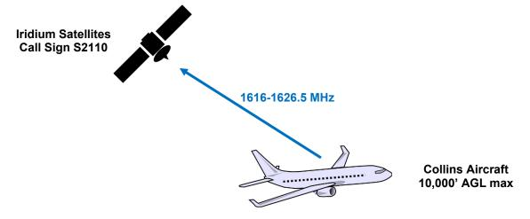
The aircraft's maximum altitude will be 10,000 feet AGL. Test duration will be approximately three (3) hours per flight.
