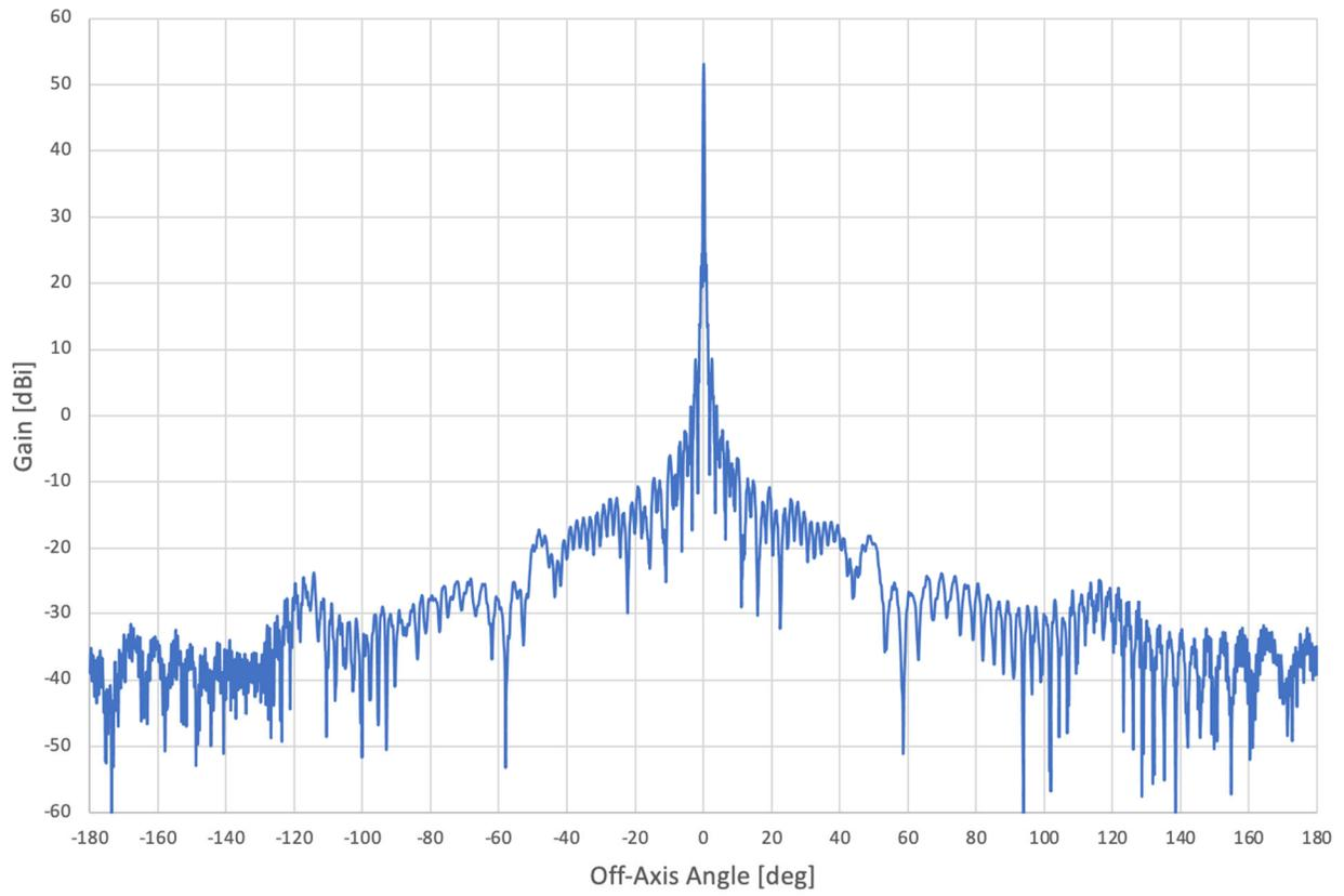
**Figure 2: TT&C Earth Station Antenna Pattern**
