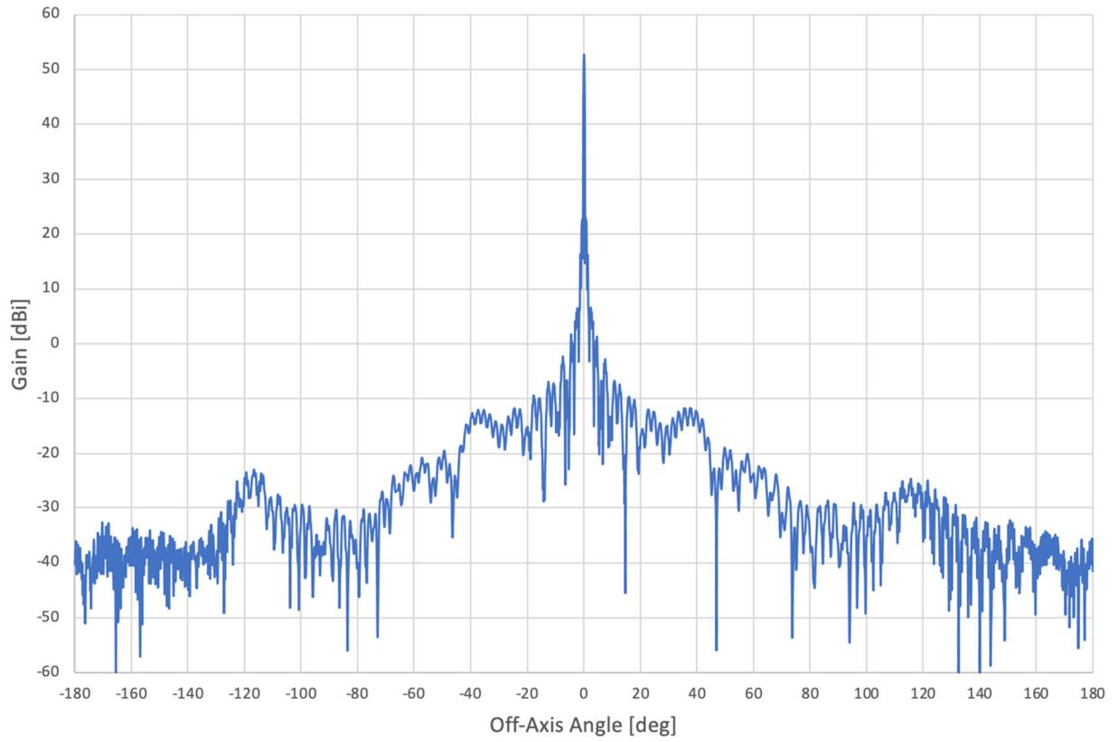
**Figure 3: Customer Terminal #1 Antenna Pattern**
