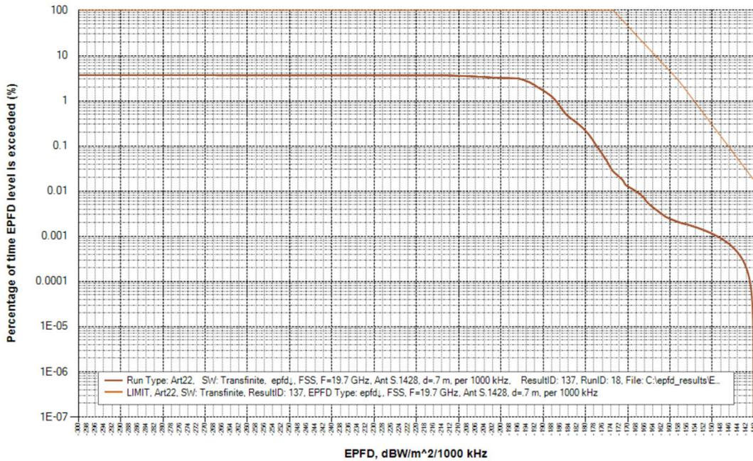
**Figure 17: Downlink EPFD, GSO Earth Station Diameter: 90cm**
