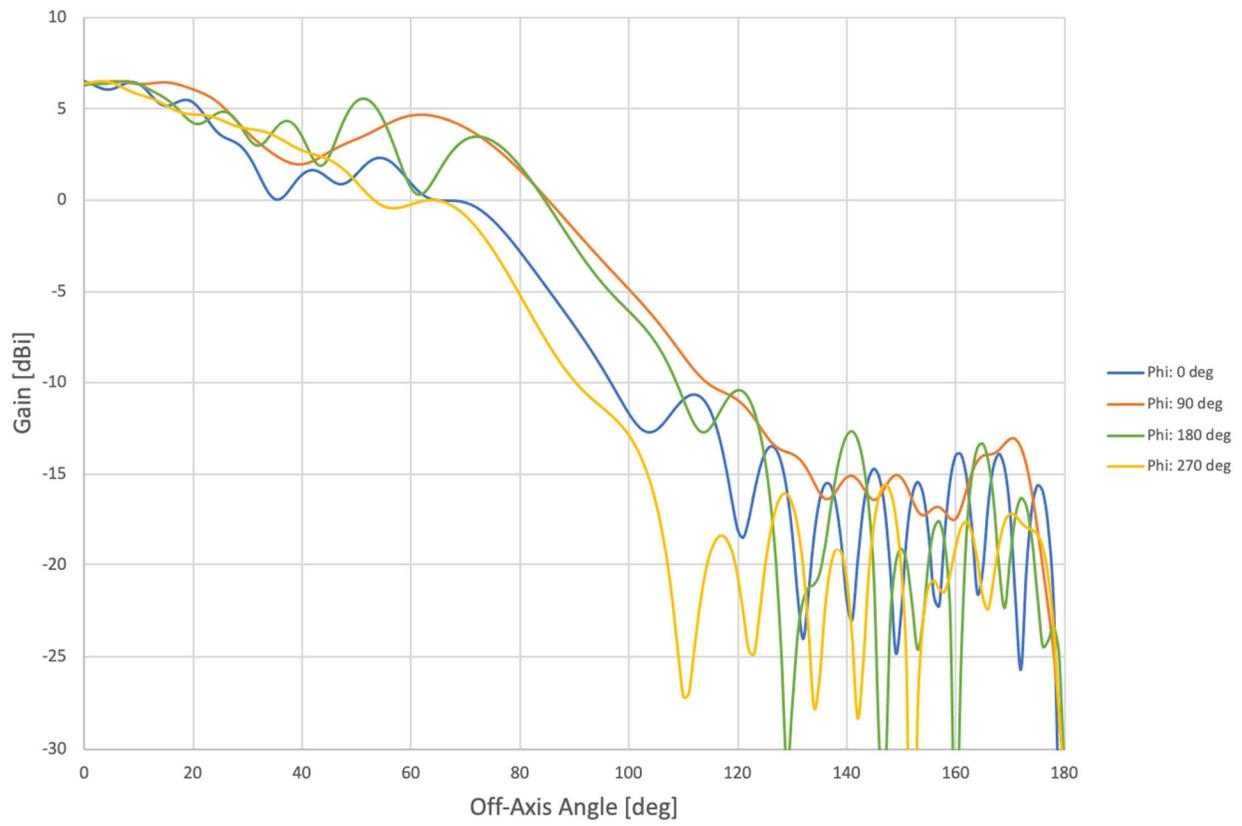
**Figure 8: Satellite L-Band Antenna Pattern**
