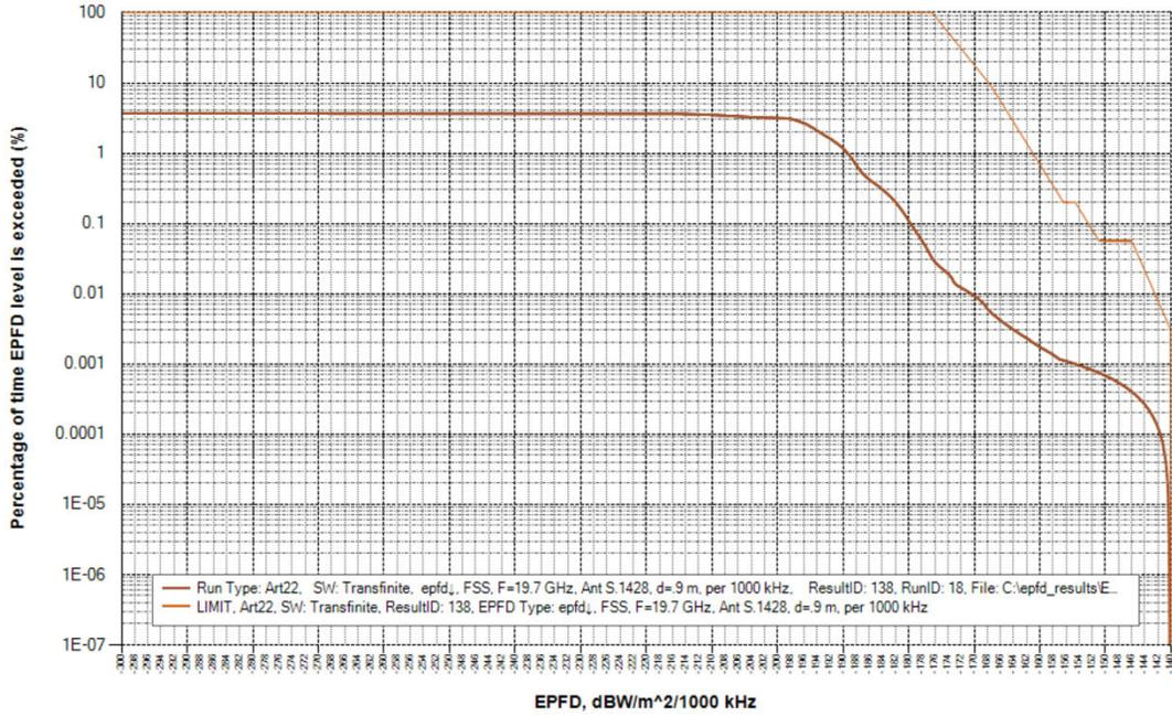
**Figure 18: Downlink EPFD, GSO Earth Station Diameter: 2.5m**
