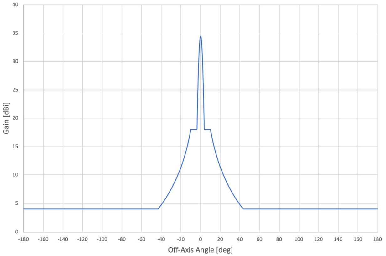
**Figure 5: Satellite Gateway Beam Antenna Pattern**
