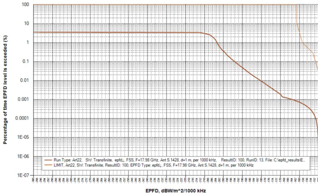
**Figure 13: Downlink EPFD, GSO Earth Station Diameter: 2.0m**
