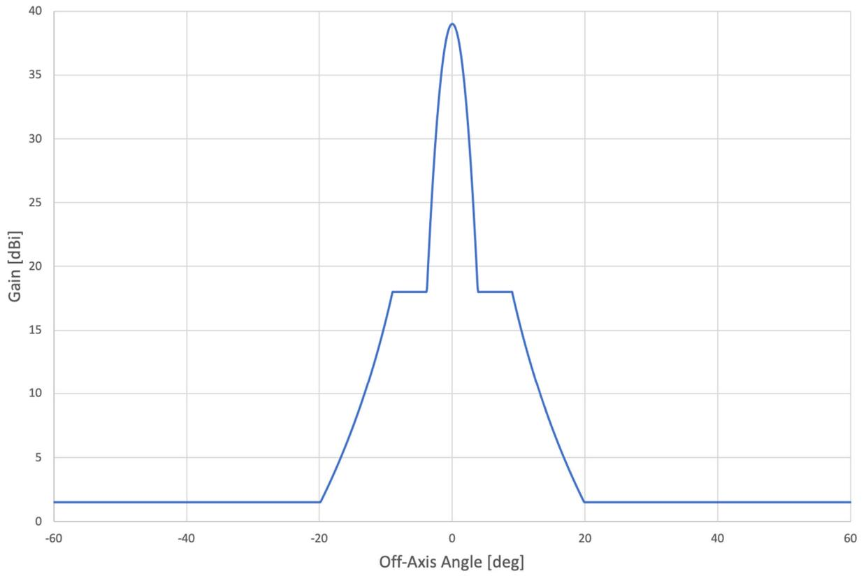
**Figure 7: Satellite TT&C Antenna Pattern**
