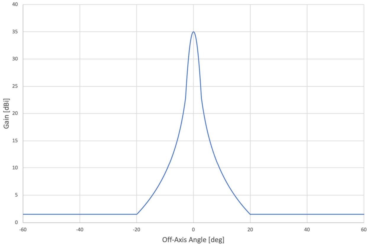
**Figure 6: Satellite User Beam Antenna Pattern**
