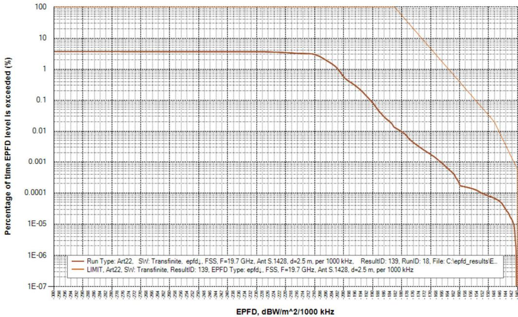
**Figure 19: Downlink EPFD, GSO Earth Station Diameter: 5.0m**
