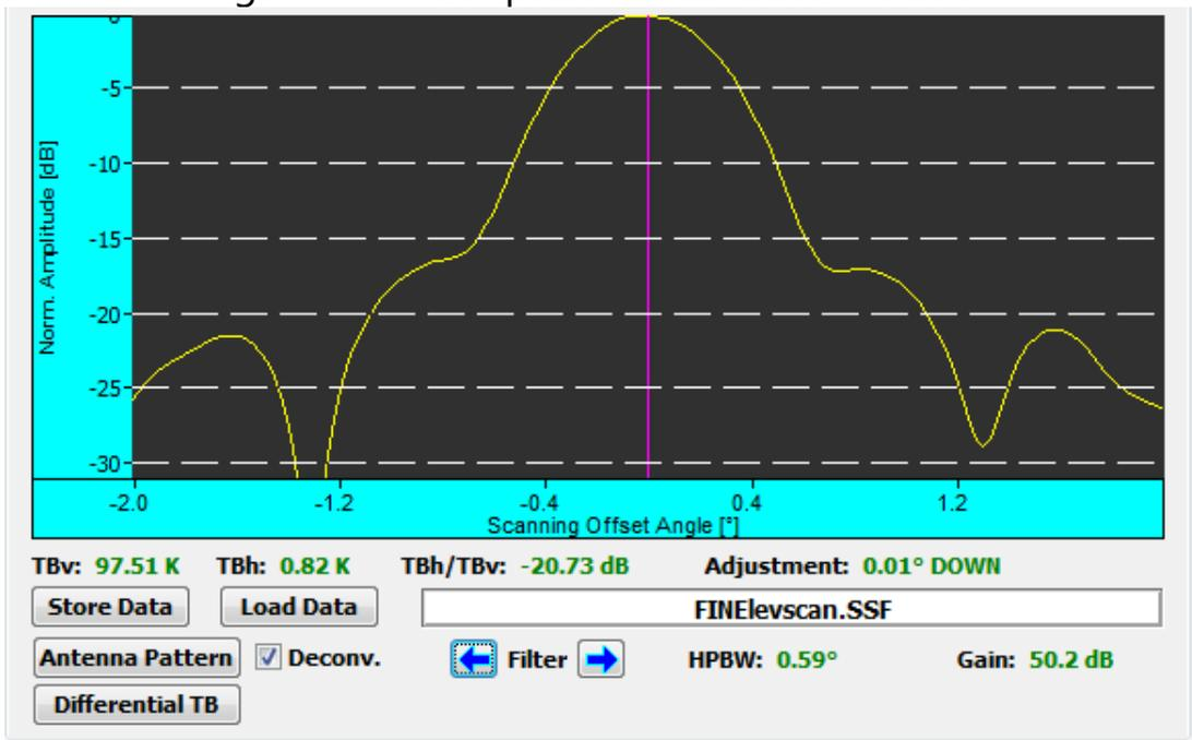
Fig. 8 – Elevation pattern after deconvolution
