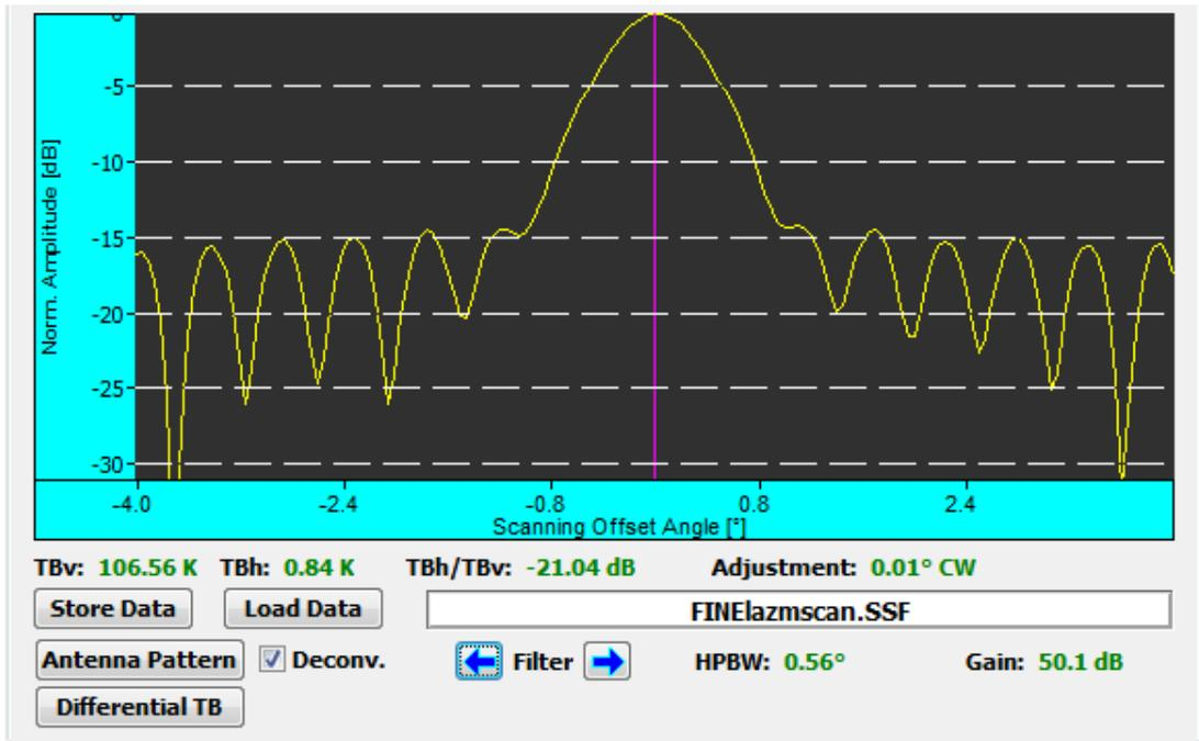
Fig. 7 – Azimuth pattern after deconvolution
