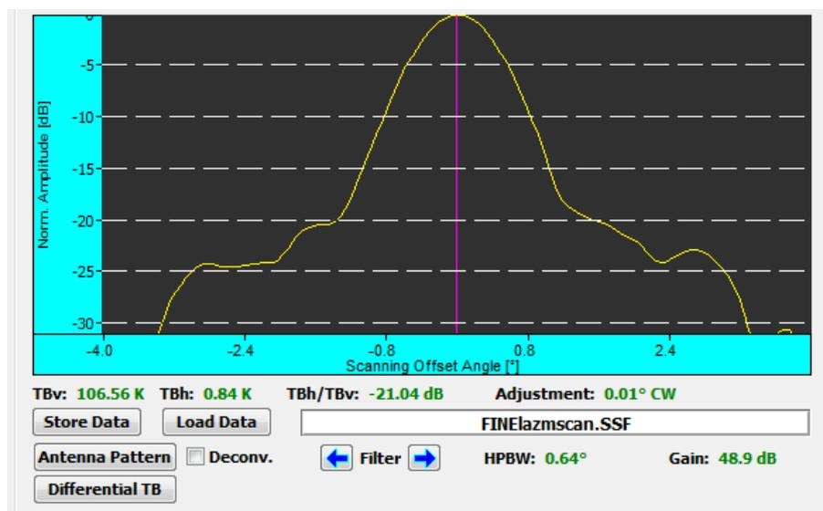
Fig. 5 – Azimuth pattern without deconvolution
