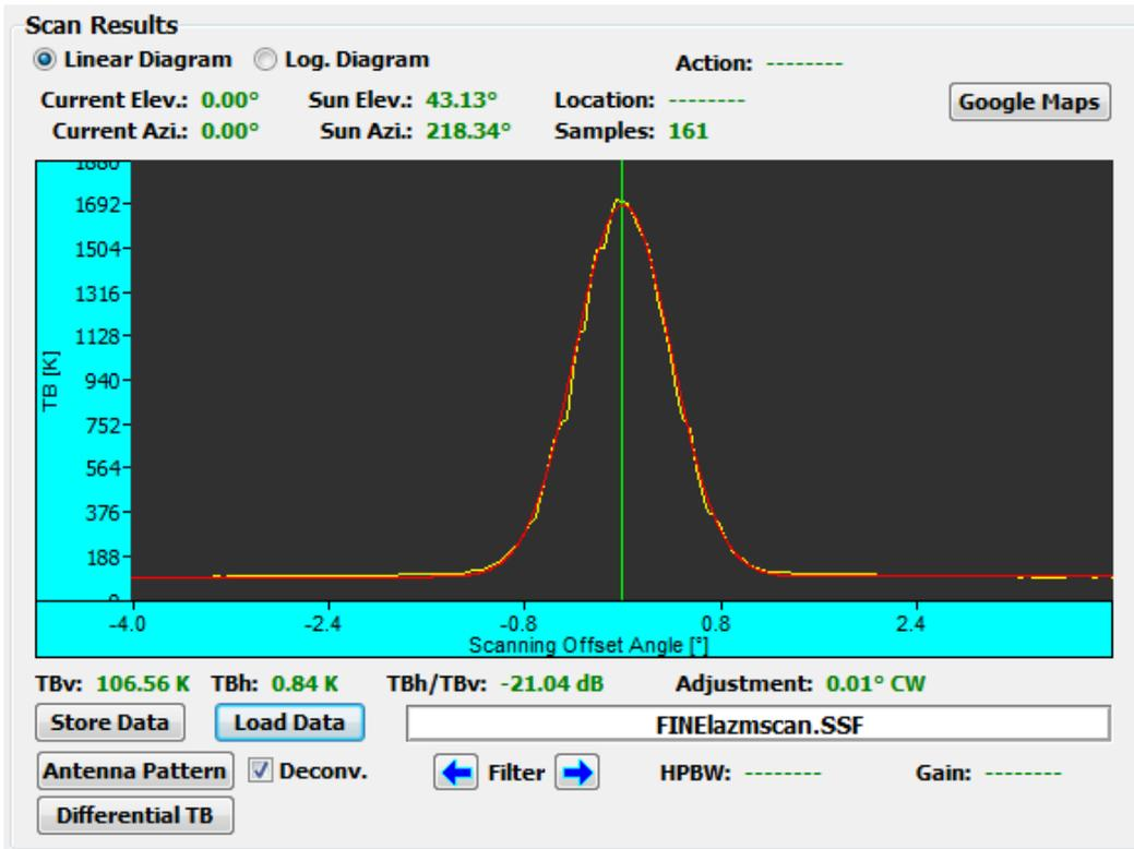
Fig. 3 – Azimuthal solar scan. Measurements are shown by the yellow line. The red line represents a Gaussian approximation.
