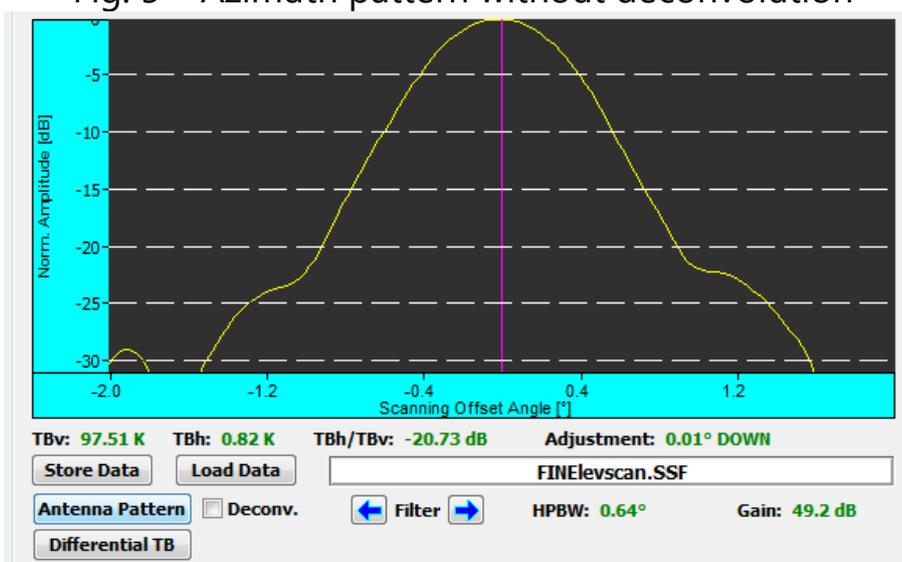
Fig. 6 – Elevation pattern without deconvolution
