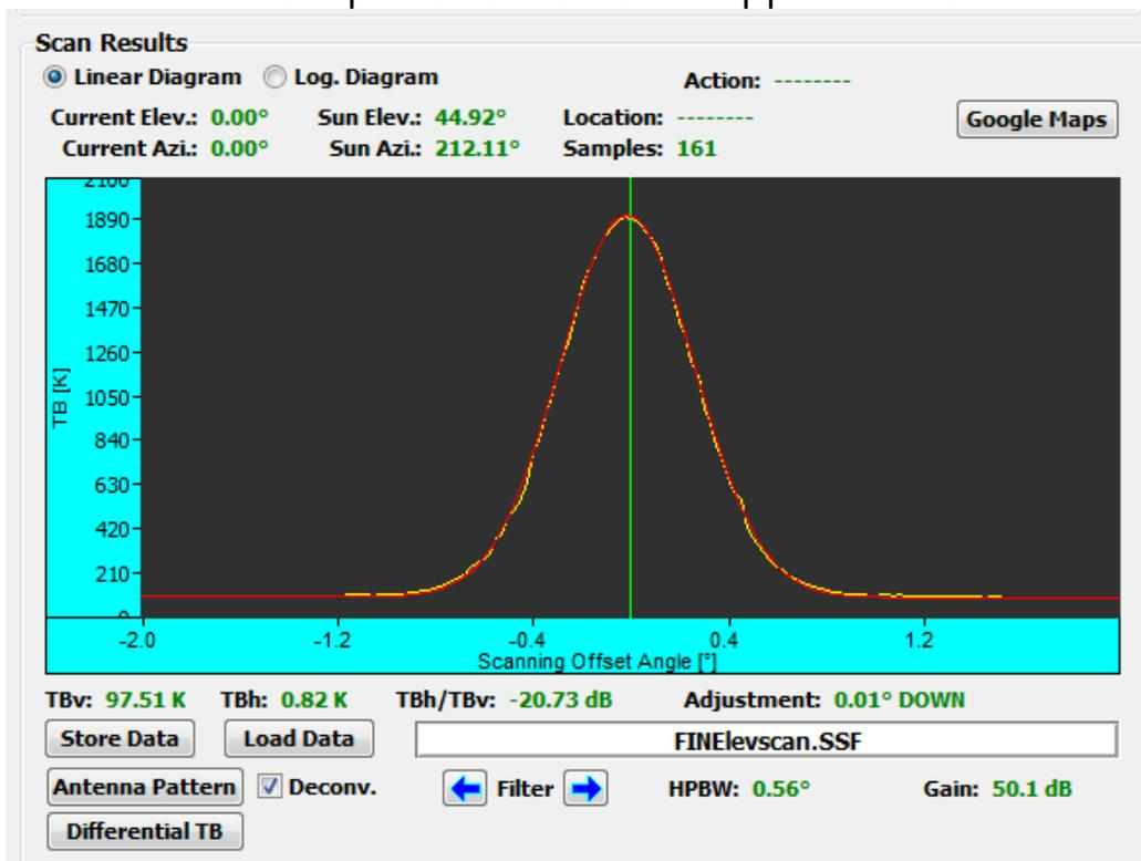
Fig. 4 – Elevation solar scan. Measurements are shown by the yellow line. The red line represents a Gaussian approximation.
