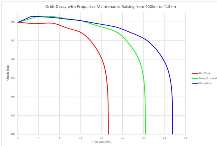
Figure 6 - Satellite lifetime after orbit raising to 415 km from 400 km with routine orbit maintenance
