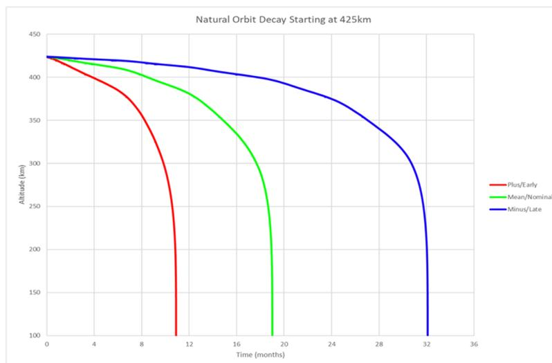
Figure 4 - Natural deorbit time (without propulsion) for the BW3 satellite
