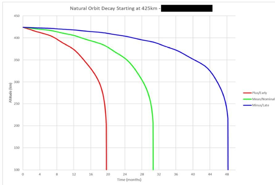
Figure 7 - Orbital decay of BW3
