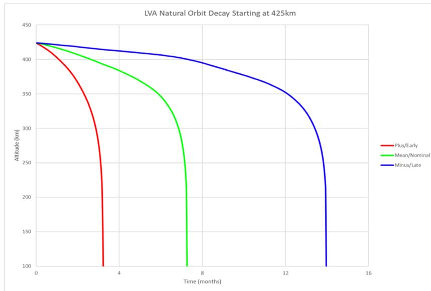
*Figure 5 - Natural deorbit time of the launch vehicle adapter*
