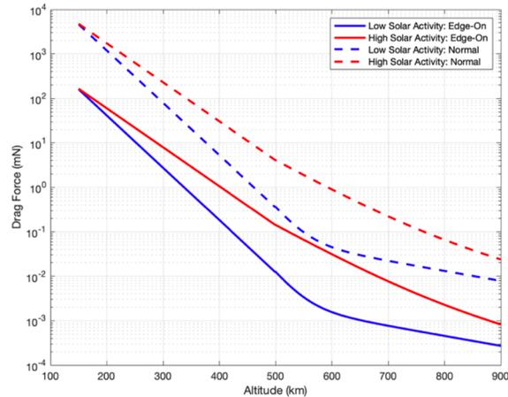
Figure 2: Atmospheric drag on BW3 satellite as a function of orbital altitude.
