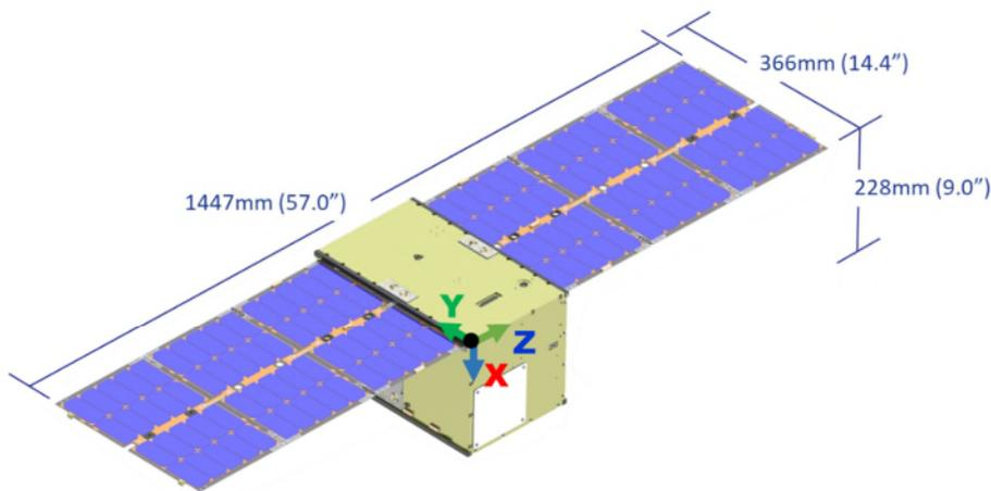
Figure 2-2: LINUS-A dimensions when the solar arrays are deployed
