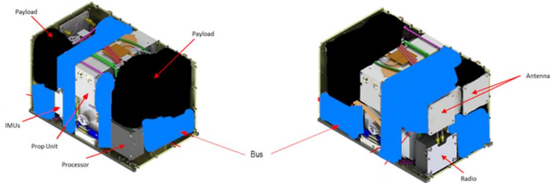
Figure 2-1: LINUS-A Interior Component View
