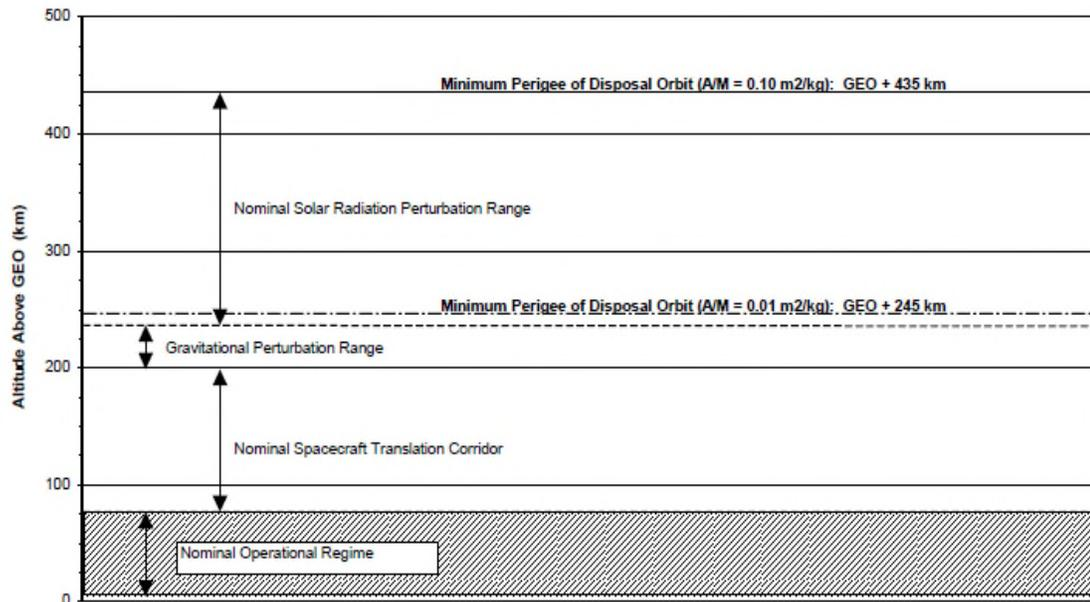
Figure 6-1: NASA STD 8719.14b specifies the minimum perigee altitude for given area to mass ratio spacecrafts
