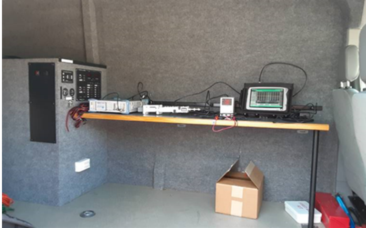
Figure 4: Interference measurement setup inside the van
