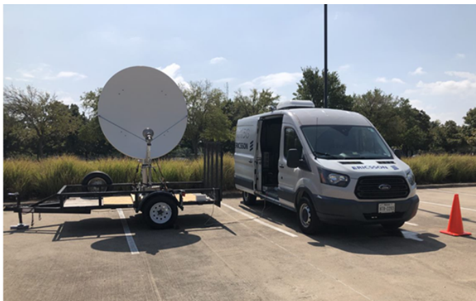
Figure 3: C band dish antenna setup for interference measurement
