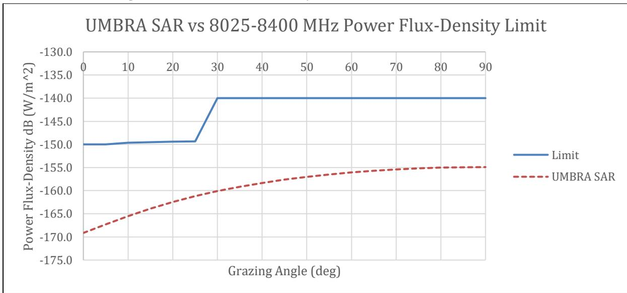
1. Power Flux Density is plotted against ITU limit
