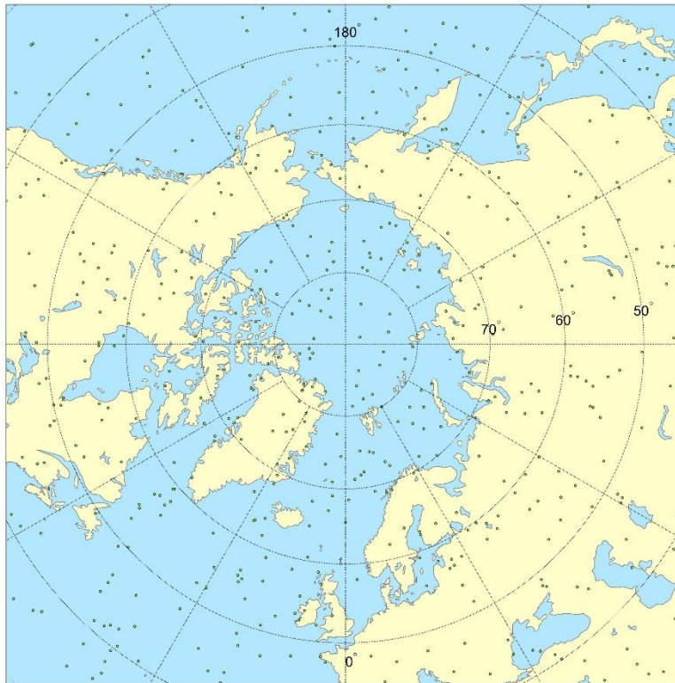
Figure 2.1-3. Arctic view of occultations from the first satellite on orbit, producing 2,160 occultations per day worldwide
