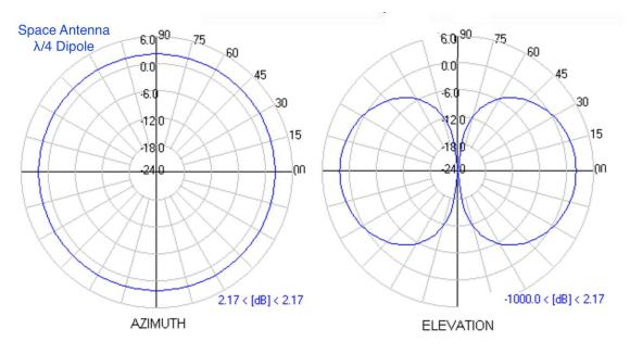
Figure 2: Space BEE (satellite) Transmit and Receive Antenna pattern.
