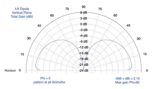
Figure 3: Ground Station Transmit and Receive Antenna pattern.
