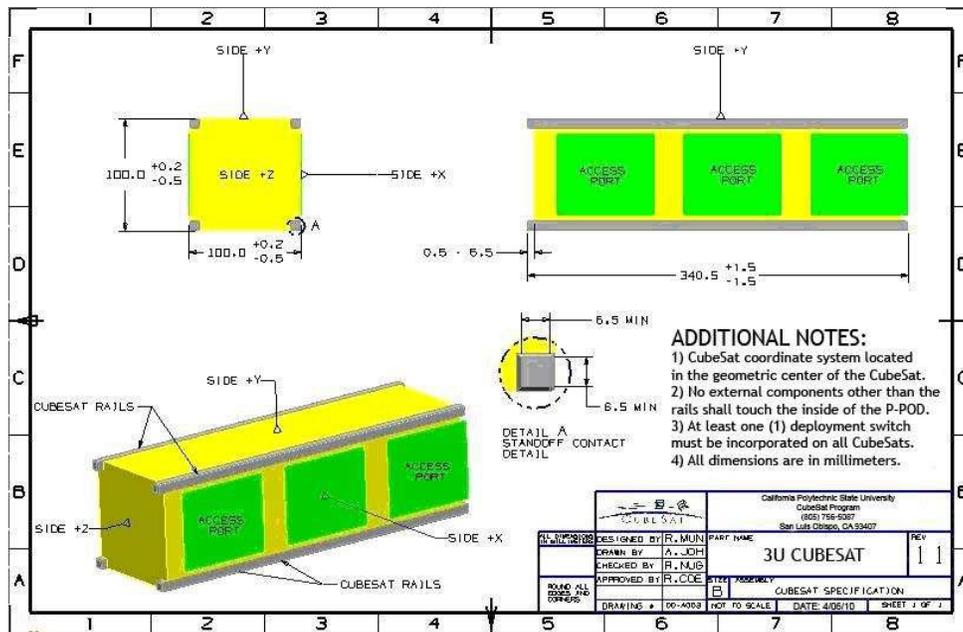
Figure 6: 3U CubeSat Specification
