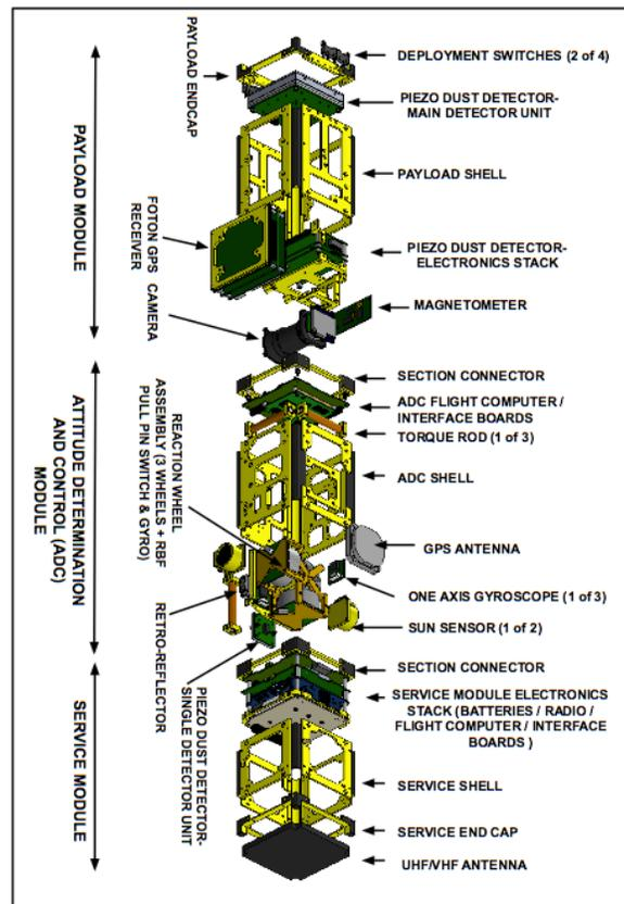
**Figure 2: ARMADILLO Expanded View (Not Showing Solar Panels)**
