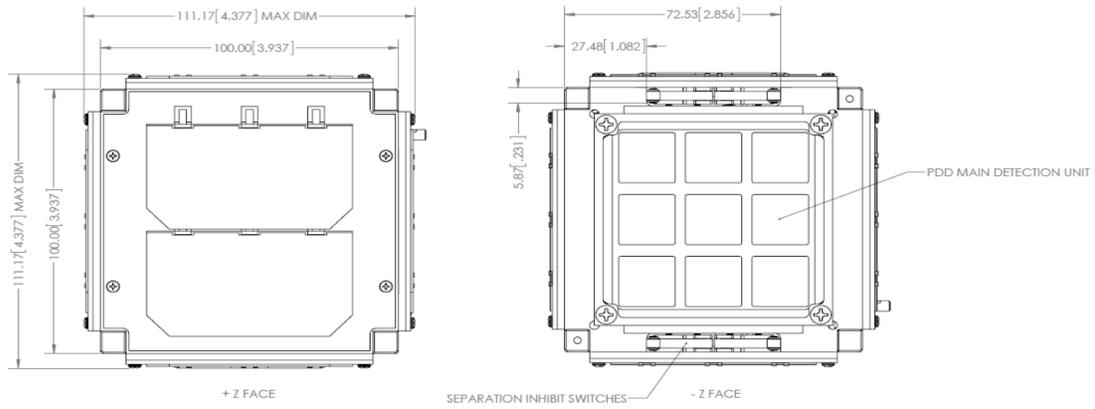
Figure 8: ARMADILLO Width Dimension (mm)
