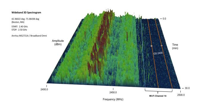
**Figure 2:** 3D Spectrographic View of 2.4 GHz Band – An 802.11 enabled TLPS will straddle the Big LEO MSS terrestrial band (2483.5 – 2495 MHz) and a generally unused portion of the upper ISM band (2473 – 2483.5 MHz). In most environments, MSS terrestrial spectrum exhibits extremely low interference levels, while the upper ISM band contains only transient low power Bluetooth emissions.
