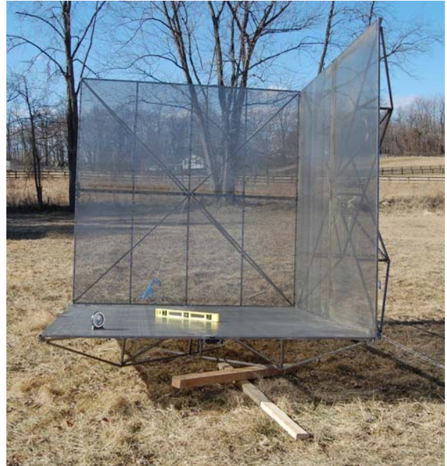
Fig-7 A P-band 2.2 m trihedral calibration target.
