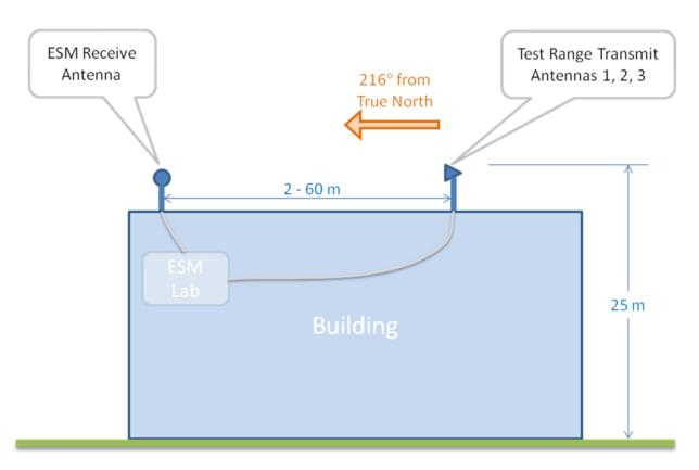
NOTE: Drawing not to scale, and rooftop metal structures higher than 25m that provide shielding to the North, East, and West are not shown
