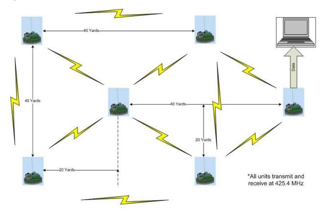
iNtelli-Sense System Demonstration set up.
