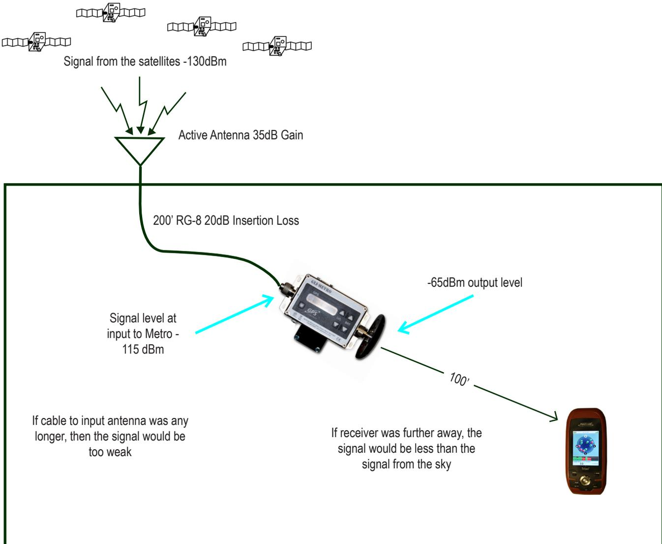
The length of the cable and the type of cable, can affect the dynamic range of the GLI-METRO (or any GPS device). The dynamic range is essentially the range of signal levels over which it can operate. The low end of the range is governed by its sensitivity. While at the high end, it is governed by its overload or strong signal handling performance.
