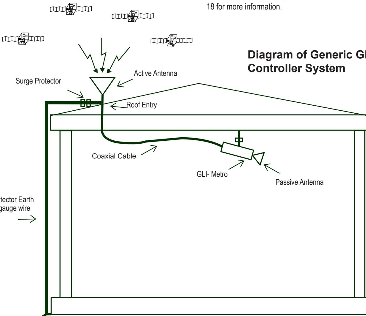
**Diagram of Generic GPS Smart Controller System**
