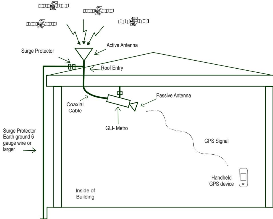
1. Mount the Receive Antenna on the roof at the location with the clearest view of the sky (this may not be the highest point).
