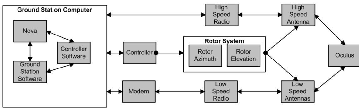
Figure 6: Component Diagram of Ground Station
