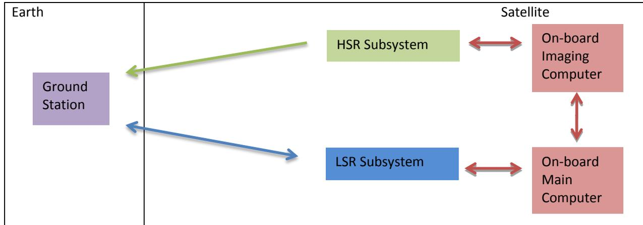
**Figure 5: Telecom System Communication Flowchart**
