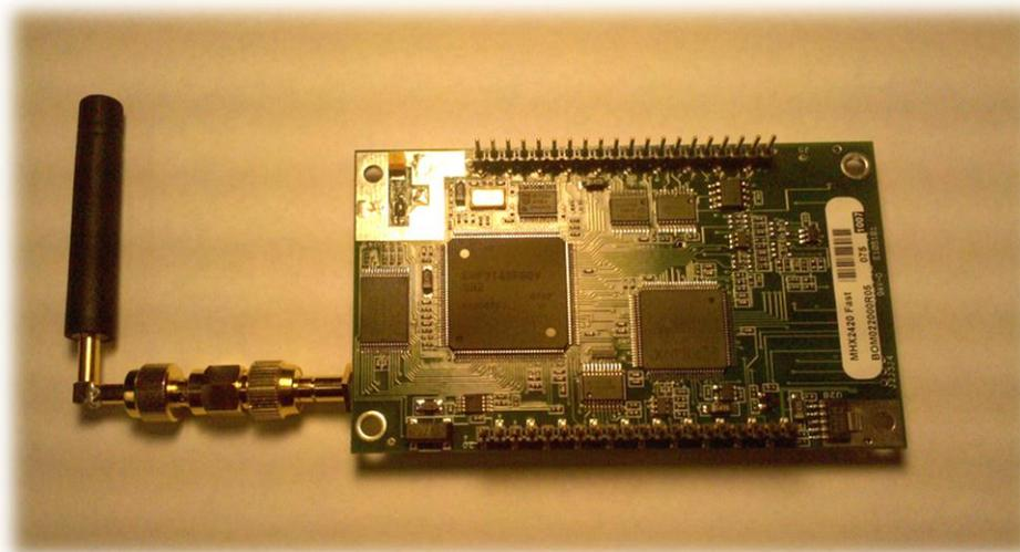
Figure 3: MHX-2420 High Speed Radio
