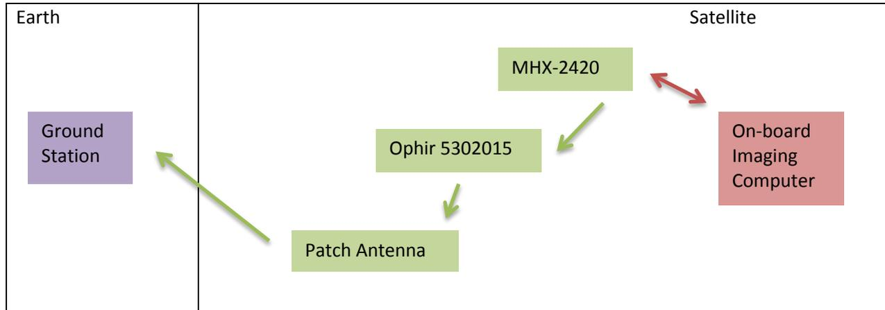
**Figure 4: HSR Communication Flowchart**
