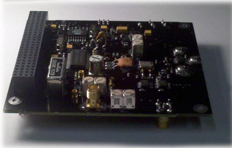
**Figure 1: ISIS TRXUV Low Speed Radio**
