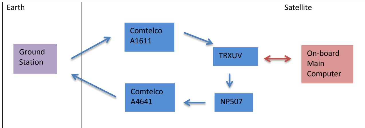
Figure 2: LSR Communication Flowchart
