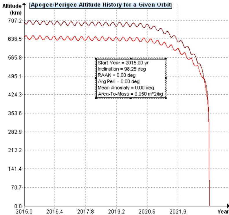
**Figure 8. Orbital Lifetime of EduSat following deorbit device deployment is less than 9 Years.**
