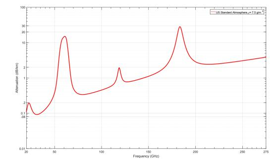
Fig. 1 Specific Attenuation Due to Atmospheric Gases
