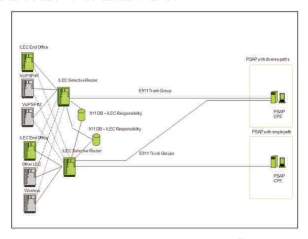
Figure 1: Enhanced 911 (E911) Network Architecture<sup>16</sup>
